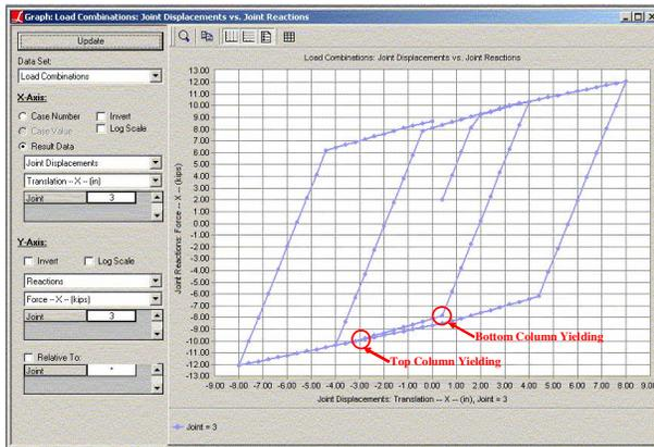
Figure 8. Force-displacement plot under cyclic loading
