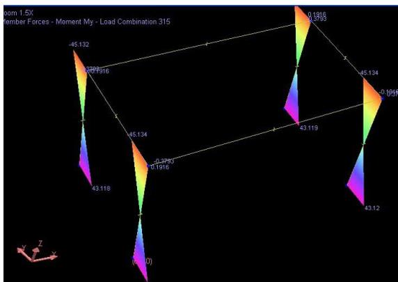
**Figure 19. Weak axis moment diagram**
