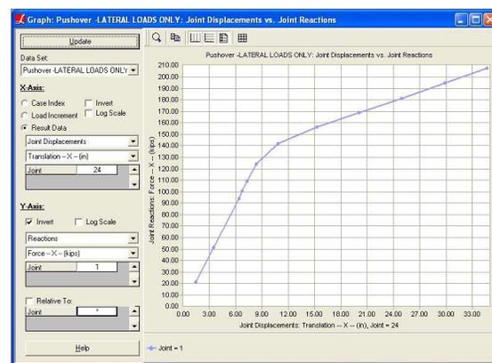
Figure 25. Base shear-root displacement plot
