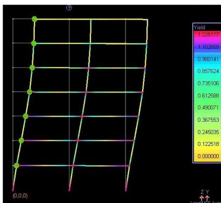
Figure 24. Displaced shape and yield function plot
