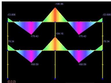
Figure 27. Moment diagram before column removal
