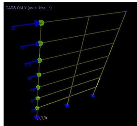
Figure 23. Example structure and load profile for pushover analysis
