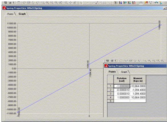
Figure 6. Spring curve for connection-beam end spring
