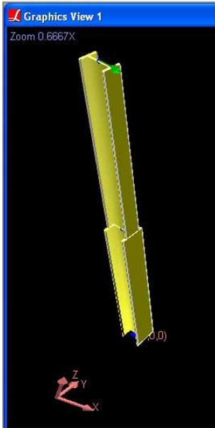
**Figure 4. Cantilever modelled with two connection-beams**
