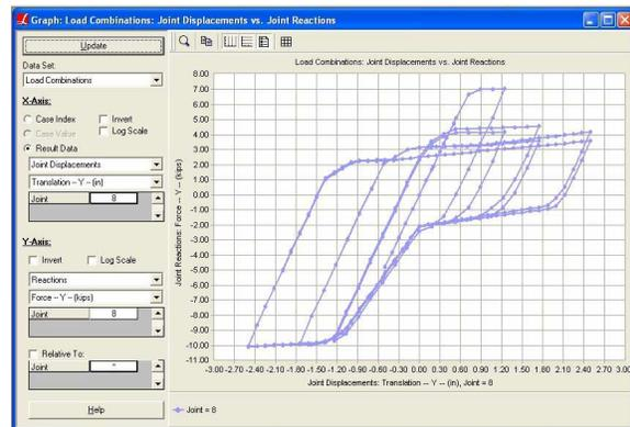
Figure 14. Force-displacement plot in the y-direction
