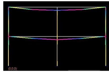
Figure 29. Yield diagram after member removal
