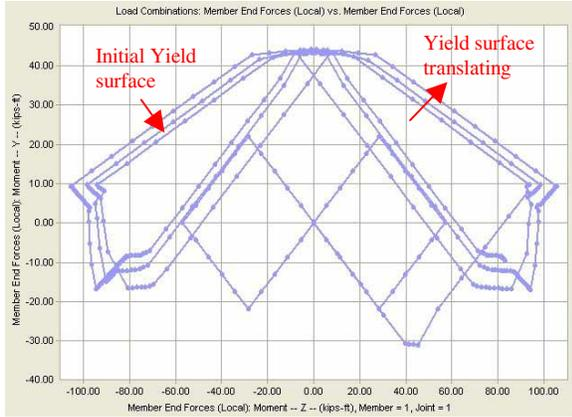
**Figure 15. Weak and Strong-axis moments in the bottom cross-section of element 1**
