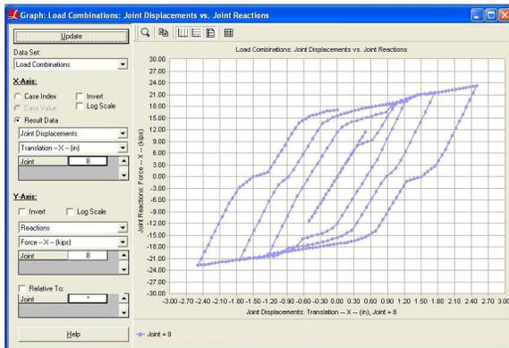
Figure 13. Force-displacement plot in the x-direction
