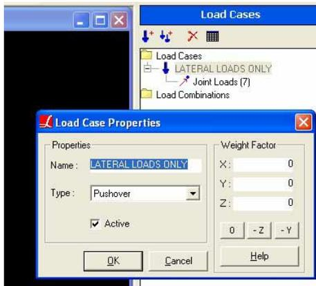
Figure 22. Pushover load-case configuration
