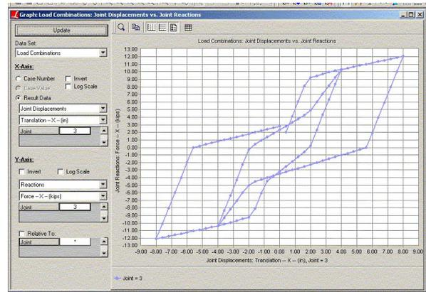
Figure 9. Force-displacement plot with slip behavior
