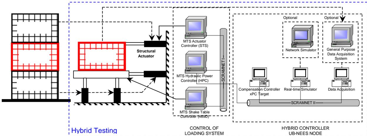
Figure 2. Schematic of Real-time Dynamic Hybrid Test System
