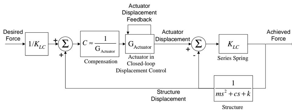
Figure 10. Block diagram of proposed force control
