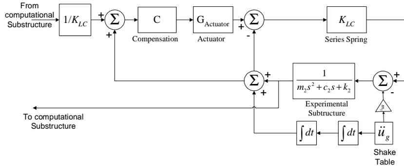
Figure 18. Control scheme for two story hybrid test
