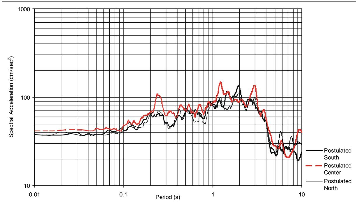
**Fig. 15 Response spectra of the synthetic accelerogram station COL (Guadalajara) downhole hypothetical southern, central, and northern Mw=8.5 earthquake scenarios**
