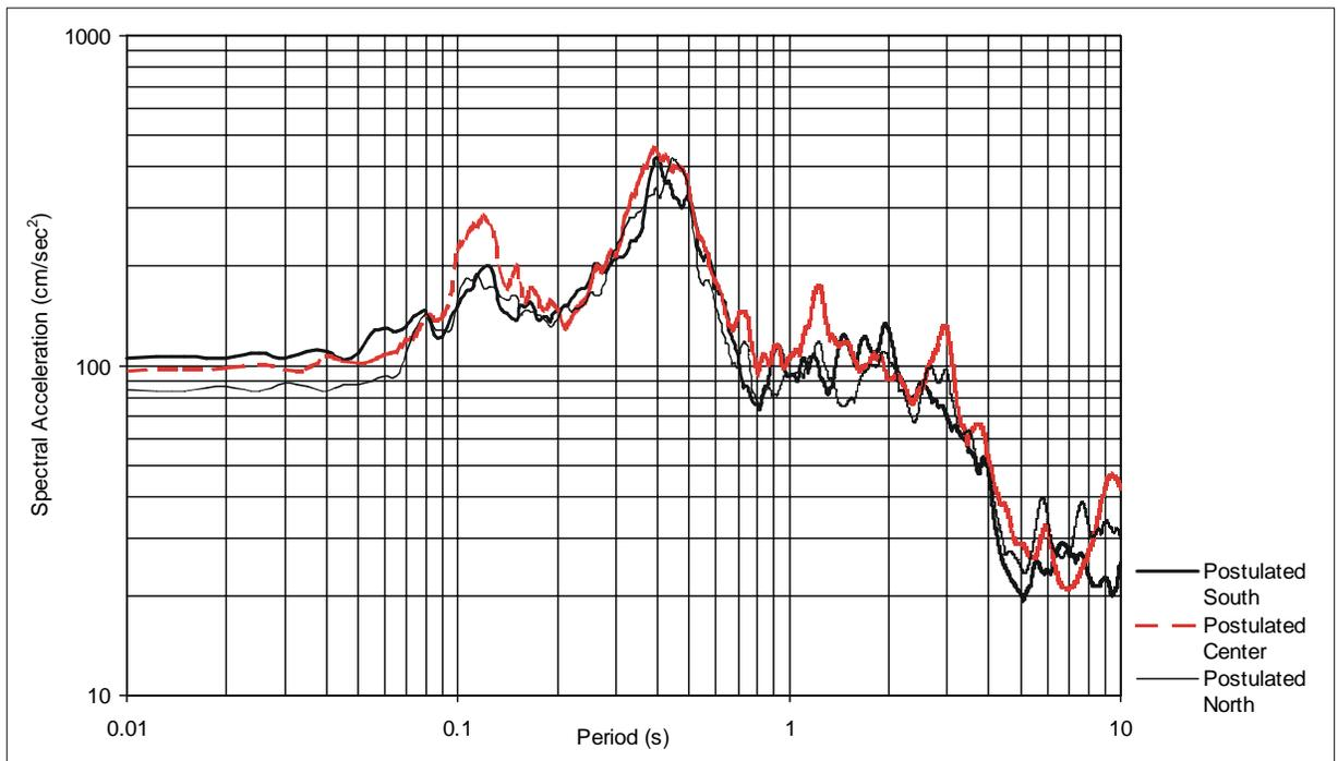
**Fig. 14** Response spectra of the synthetic accelerogram station COL (Guadalajara) surface hypothetical southern, central, and northern Mw=8.5 earthquake scenarios
