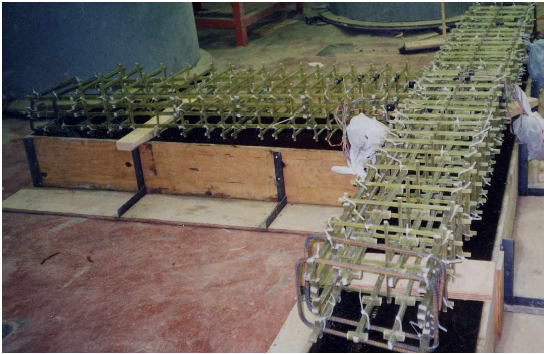
Fig. 2. View of the GFRP reinforcement cage for specimen (J4) lifted on the forms before casting.
