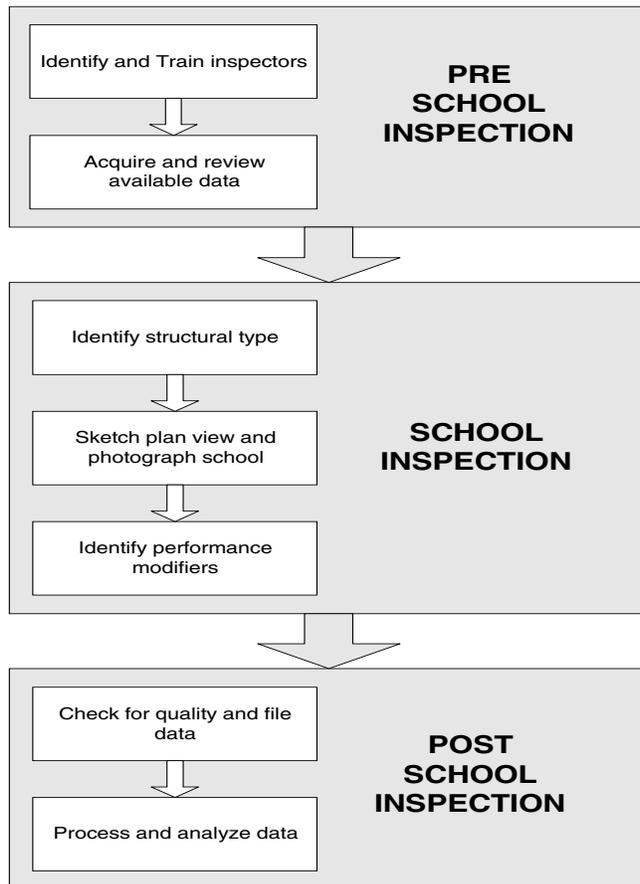
**Fig. 4 Stages of the visual inspection**
