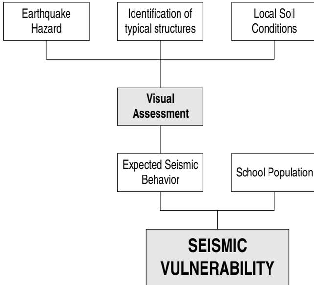
**Fig. 3 Methodology for assessing seismic vulnerability**
