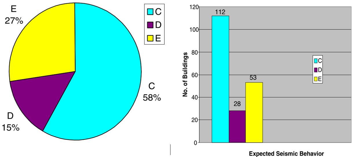
**Fig. 14** Expected earthquake behavior for C3 buildings
