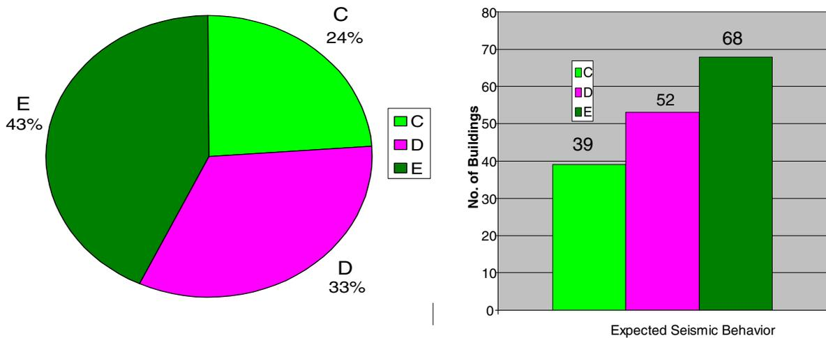
**Fig. 15** Expected earthquake behavior for CM buildings
