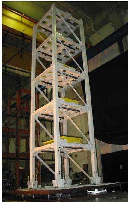
**Figure 5: Photograph of tested five-story isolated model structure on seismic simulator of the University at Buffalo**
