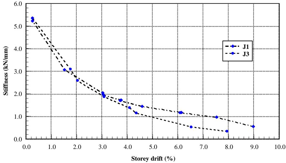
**Figure 9. Secant stiffness-displacement ductility factor for the tested specimens.**
