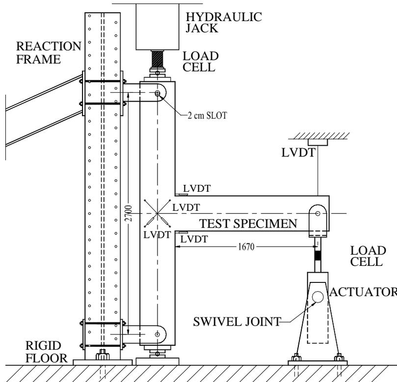
Figure 3. Test setup.
