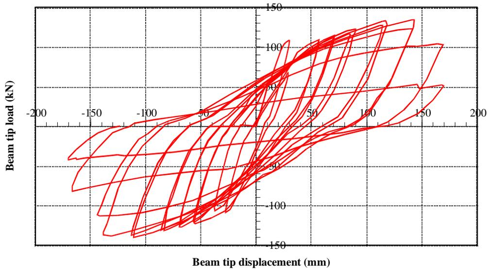
**Figure 4. Load displacement relationship for NC specimen *J1*.**
