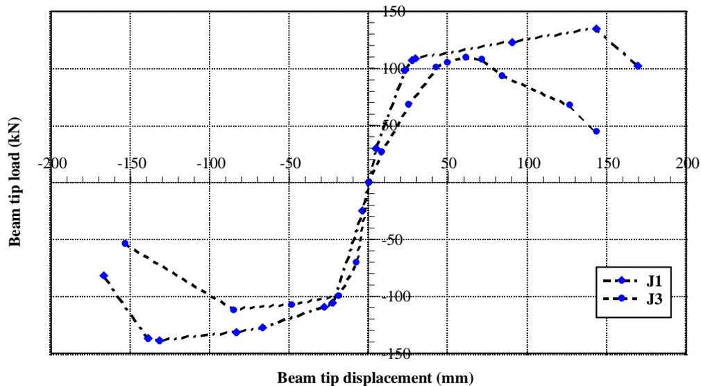
Figure 7. Load-displacement envelopes for the tested specimens.
