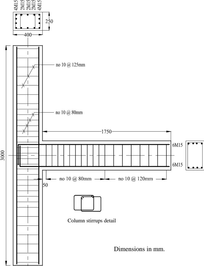
**Figure 1. Reinforcement details for the specimens.**
