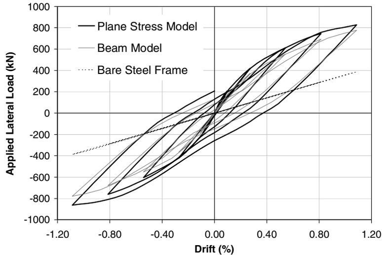
**Figure 14: Hysteretic response of a single-bay steel frame with and without the retrofit system.**
