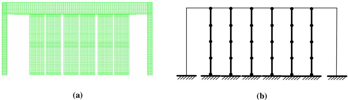
**Figure 13: Single-bay finite element models with the retrofit system; plane stress finite element model (a) and beam element model without panel springs (b)**
