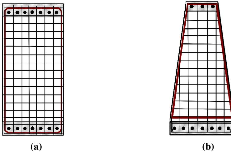
**Figure 3: Panel geometry and reinforcement for rectangular panels (a) and tapered panels (b).**
