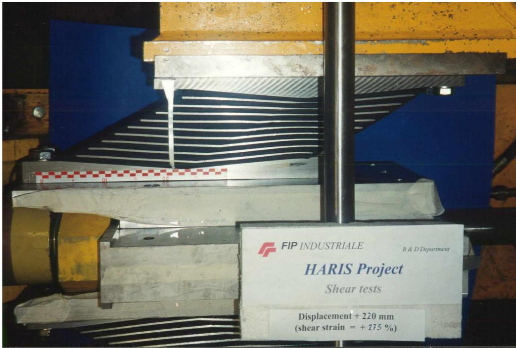
**Figure 8 – Bending deformation of steel plates subjected to high shear strains.**
