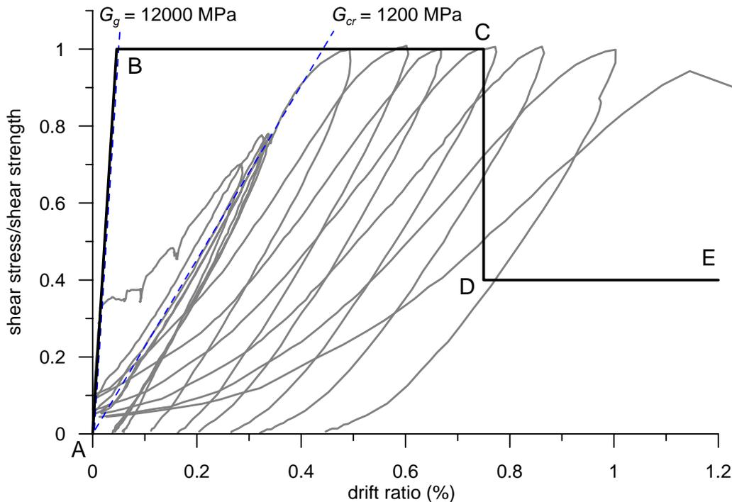
**Figure 1 FEMA 356 generalized load-deformation function for shear walls compared to results from a membrane element test (Stevens et al. [3])**
