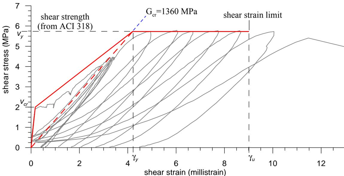
**Figure 6 Proposed load-deformation curve for non-linear static analysis (shown for membrane element test SE8, Stevens et al. [3])**
