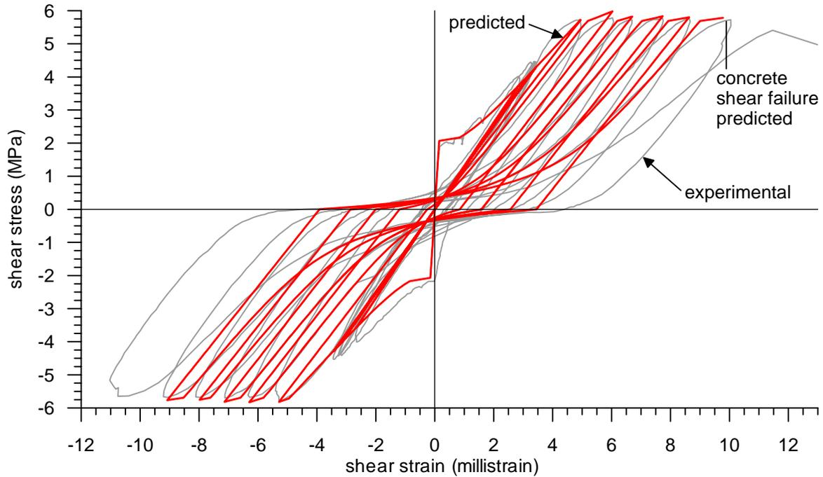
**Figure 3 Comparison of General Model prediction (Gérin [9]) and the results from a membrane element test (Stevens et al. [3])**
