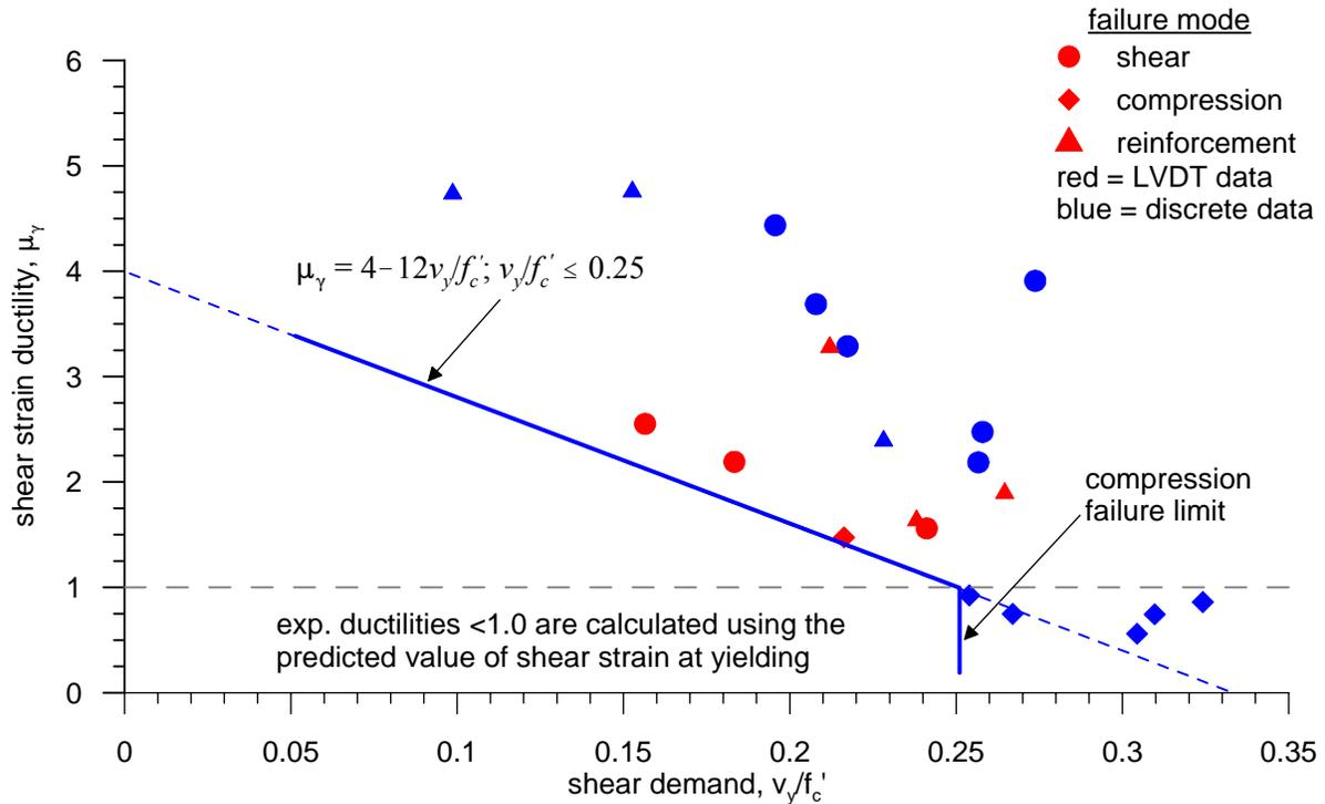
**Figure 5 Proposed shear strain ductility**
