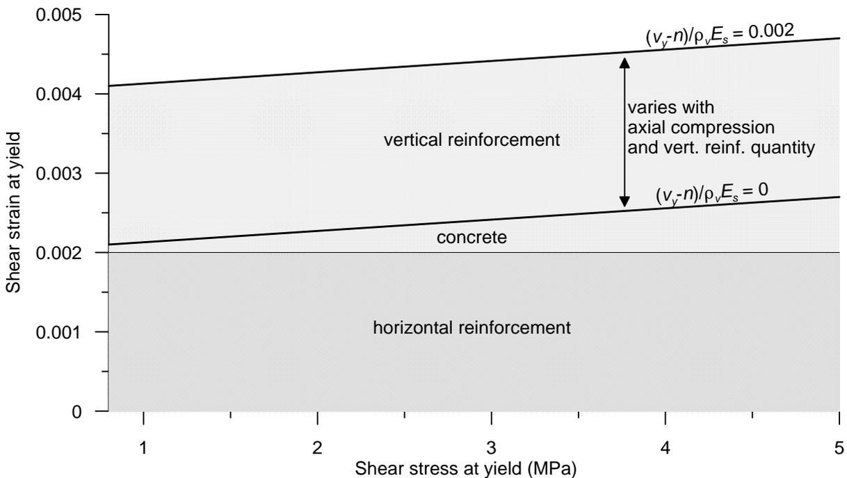
**Figure 4 Contributions to shear strain at yield for typical shear walls**
