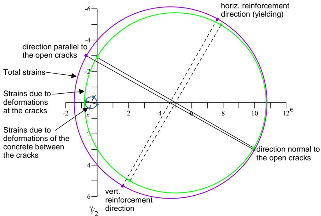
**Figure 2 Crack and concrete components of total strains for a point after yielding of the weak reinforcement**
