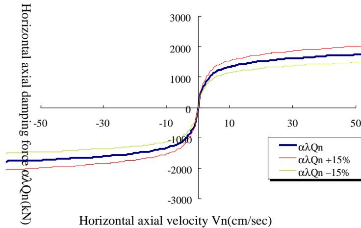
Figure 6. Relationship between axial velocity  $V_n$  and damping force  $\alpha\lambda Q_n$
