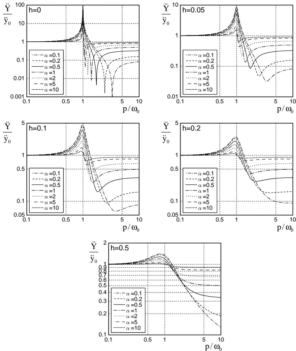
Figure2. Response magnification of single lumped mass with added mass, m
