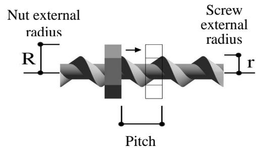
Figure 5. Relation of Screw pitch and Nut
