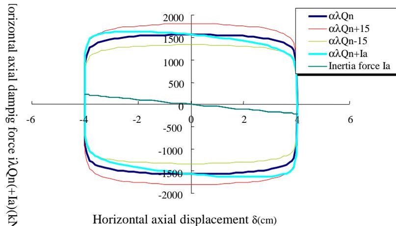
Figure 7. Relationship between axial displacement  $\delta$ -damping force  $\alpha\lambda Q_n(+I_a)$  (characteristics of steady state input wave)
