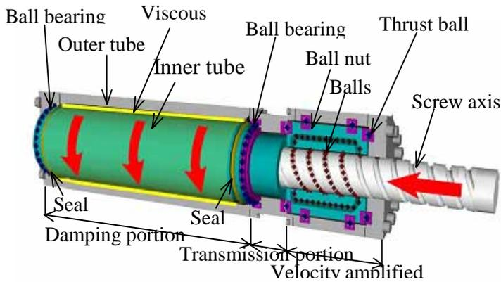
Figure 4. Gyro/Mass-Viscous damper (GMD)
