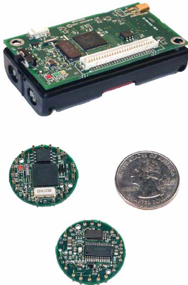
Figure 8. Berkeley-Mote (Mica2 and Mica2dot) Processor Boards.
