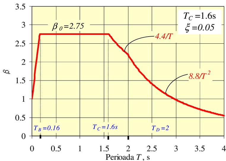
**Figure 9. Normalised acceleration response spectra for horizontal ground motion in zones characterised by control periods  $T_c = 0.7s$ ,  $T_c = 1.0s$  and  $T_c = 1.6s$ , in the P100-2003 code proposal**
