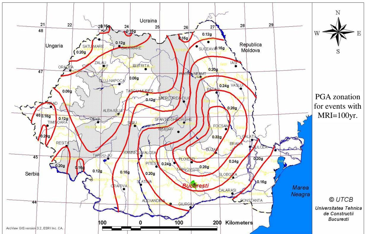
**Figure 7. The design ground acceleration for an event with  $MRI=100$  years.**
