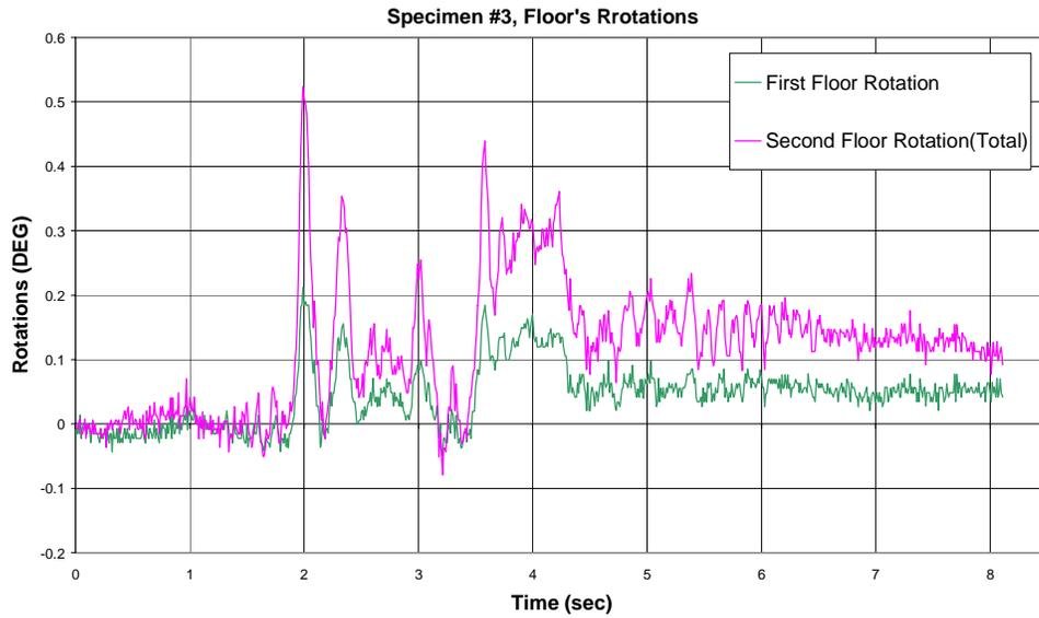
Fig. 16: Roof's rotation in Specimen #3, maximum table excitation  $9.093 \text{ m/sec}^2$
