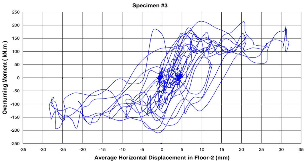
Fig. 17: Overturning moment in specimen #3, maximum table excitation  $9.093 \text{ m/sec}^2$
