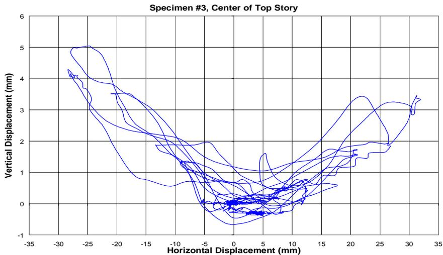
Fig. 15: Second roof vertical displacement vs. average horizontal displacement for the top story in specimen #3, maximum table excitation 9.093 m/sec<sup>2</sup>
