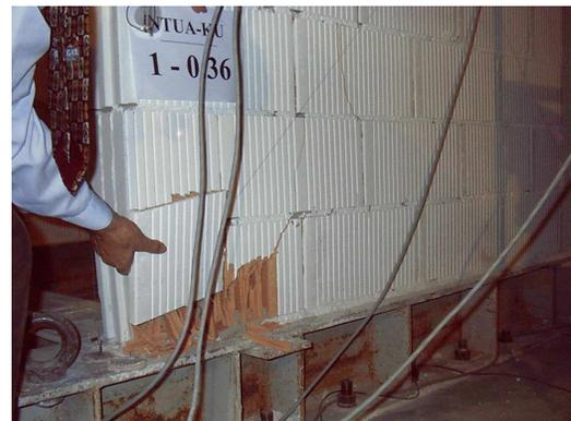
Fig. 9: Last test in specimen #1, shear failure caused collapse in first layer of main wall
