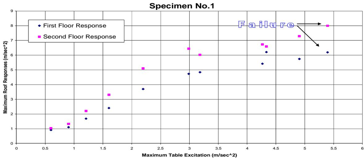
Fig. 13: Maximum table excitation vs. maximum floor responses specimen #1
