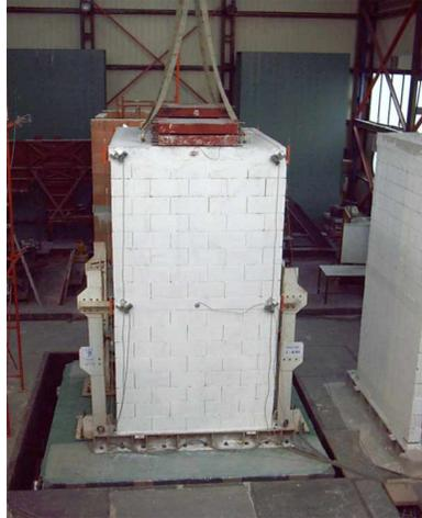
Fig. 6: Instrumentations on specimen #1 ready for testing (LVDTs & Accelerometers)
