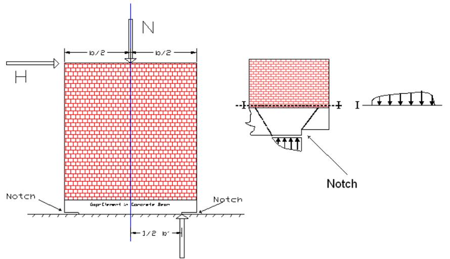
Fig. 1: Corner-Gap-Element in masonry wall
