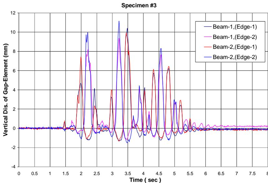
Fig. 18: Vertical opening (jumping) of Gap-Elements for specimen #3, maximum table excitation 9.093 m/sec<sup>2</sup>
