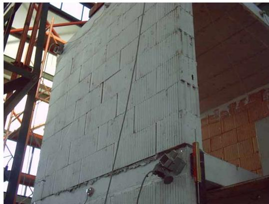
Fig. 10: Step-like diagonal crack through joints at 72 % g excitation
