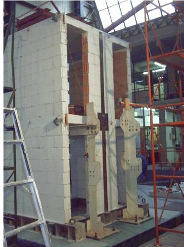
Fig. 4: Steel strip in lateral walls for prevention of out of plane failure
