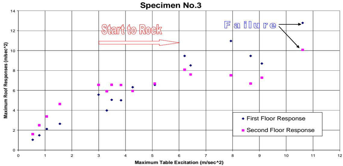
Fig. 14: Maximum table excitation vs. maximum floor responses specimen #3
