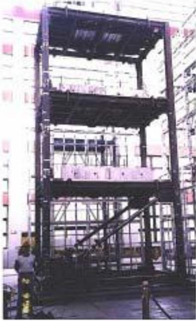
Fig. 8: 3-Story Full-Scale Building on the Shake Table of NCREE
