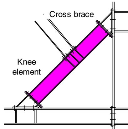
**Figure 1. Typical knee element configuration**
