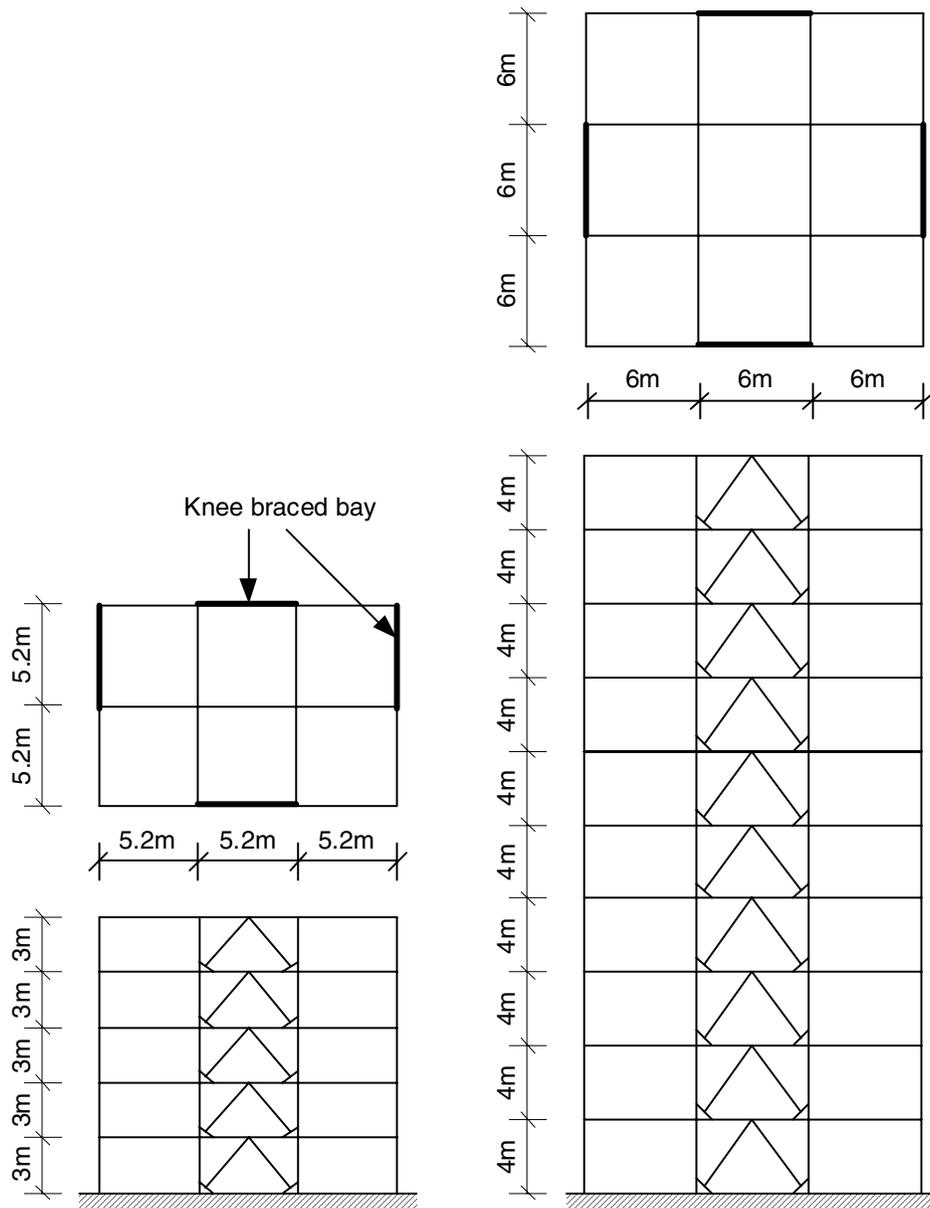
**Figure 4. Plans and elevations of the two knee-braced frames**
