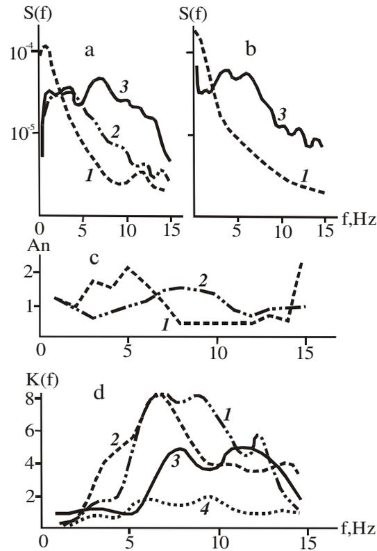
**Fig. 2. Experimental data on the spectra and relative frequency characteristics form the earthquakes recorded on rocky grounds of a different condition.**
