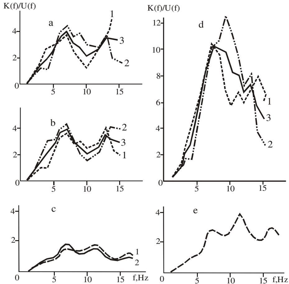
**Fig. 3. Ratios of experimental  $K(f)$  to computational  $U(f)$  frequency characteristics for rocky grounds.**
