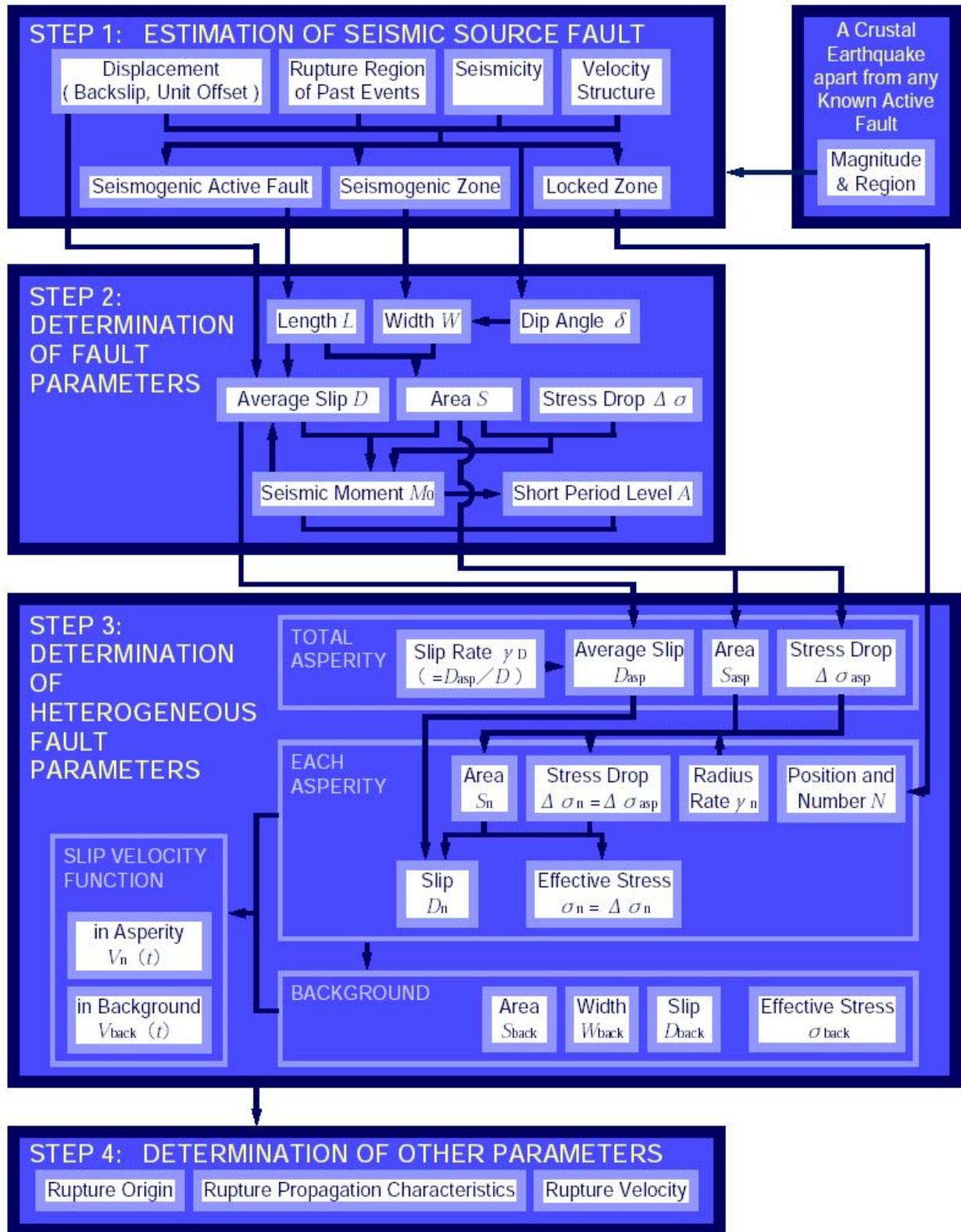
Figure 1 Procedure to Determine Characterized Fault Models of Scenario Earthquakes
