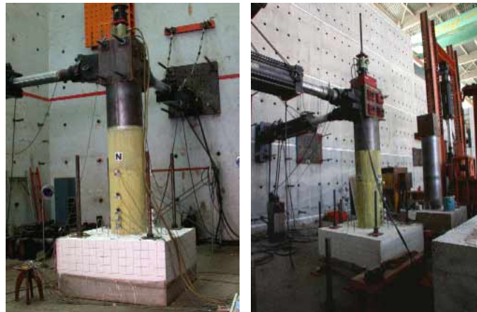
Figure 6 Installation of DSCFT piers in NTU (left) and NCEE (right)
