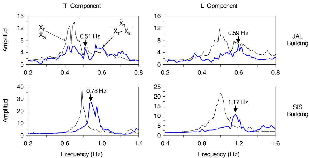
**Figure 5. Fixed-base ( $RF_s$ ) and system ( $RF_{sys}$ ) spectral ratios**
