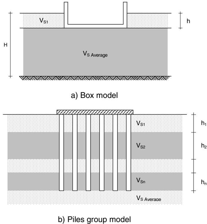
**Figure 2. Basic models for assessment of foundation stiffnesses**
