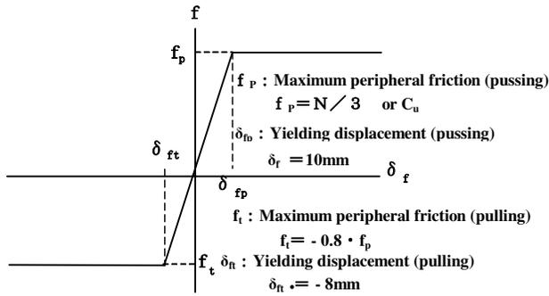
Figure12: Pile peripheral friction spring
