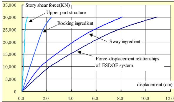
Figure17: Force-displacement relationships of ESDOF system
