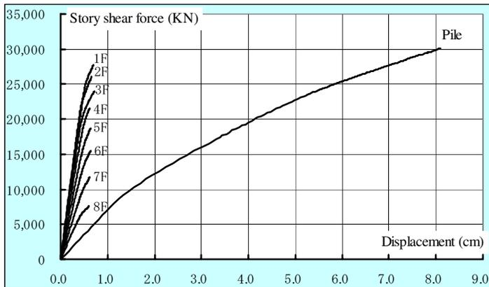
Figure15: Force-displacement curves in span direction
