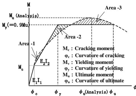
Figure10: Model of pile ( $M-\phi$  relationship)
