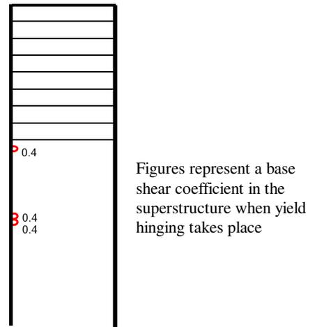
Figure16: Hinging in pile foundation monolithic model
