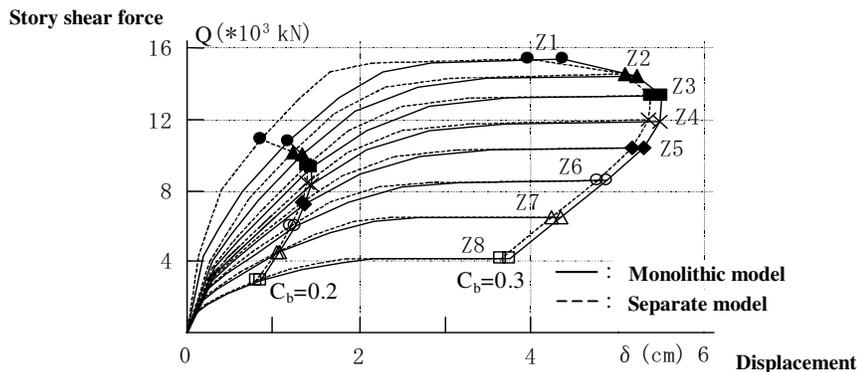
Figure14: Force-displacement curves in ridge direction
