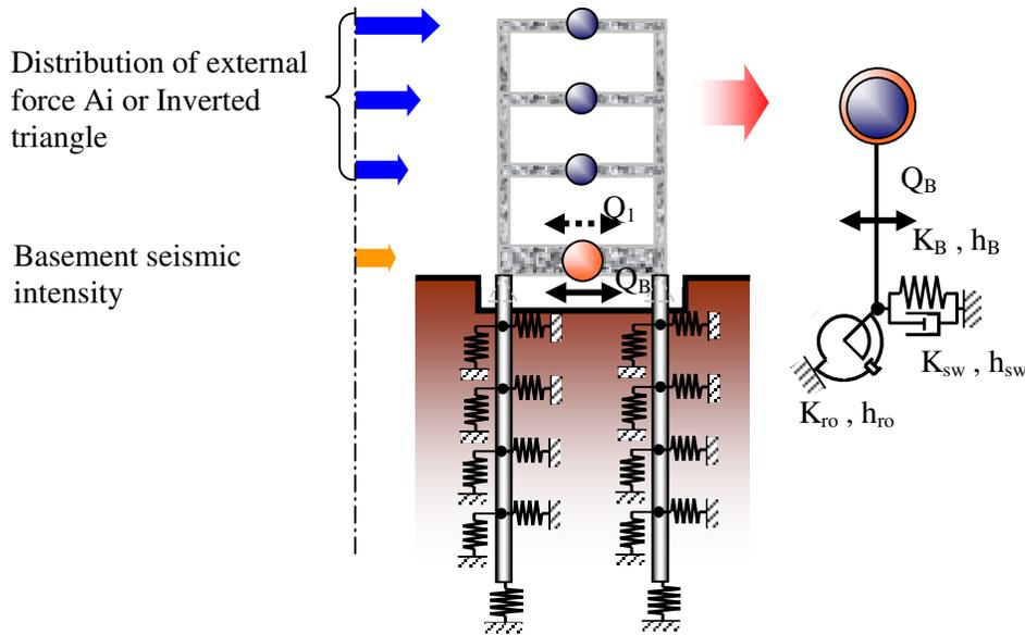
Figure3:Conversion to equivalent single-degree-of-freedom(ESDOF)system of monolithic model
