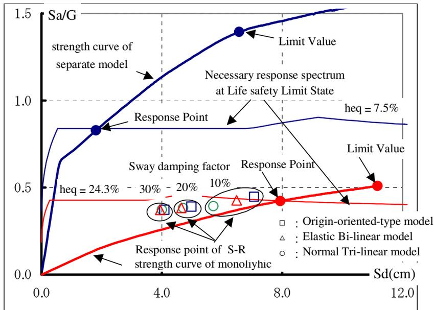
Figure19: Comparison of analysis result by the Capacity Spectrum Method and response analysis with S-R model
