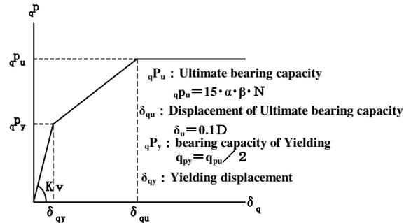
Figure13: Pile tip support spring
