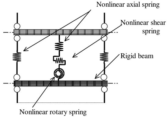
Figure9 Model of shear wall (Kabeyasawa Model)
