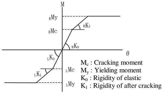
Figure8: Model of Beam
