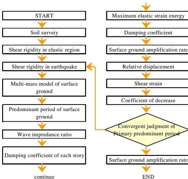
Figure1: Calculation procedure of surface ground amplification rate
