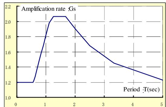
Figure2: Acceleration amplification rate to have nonlinear of surface ground  $G_s$
