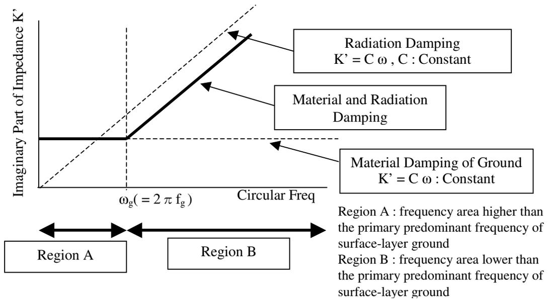
Figure4: Simplified Evaluation for Imaginary Part of Impedance
