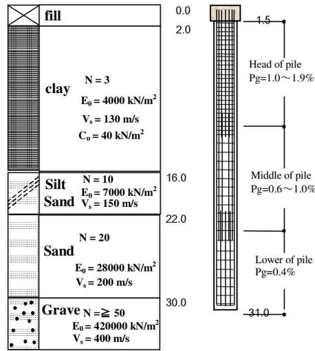
Figure6: Ground condition and model of pile
