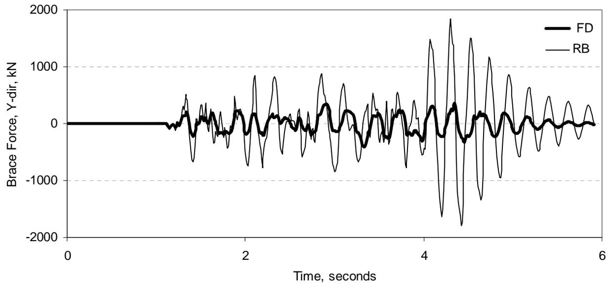
Figure 7. Time history of axial forces in 4<sup>th</sup> floor single diagonal brace
