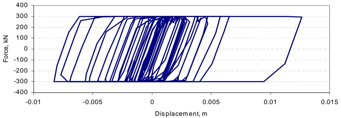
Figure 9. Hysteretic loop of friction damper
