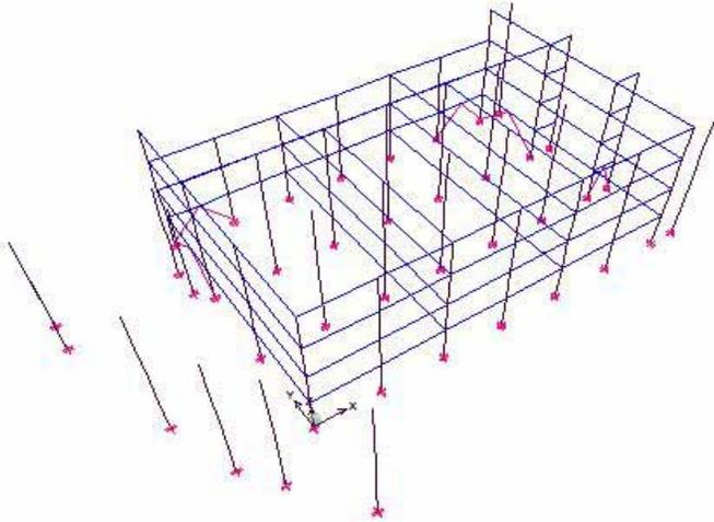
Figure 3. West Wing, 3-dimensional analytical model of building
