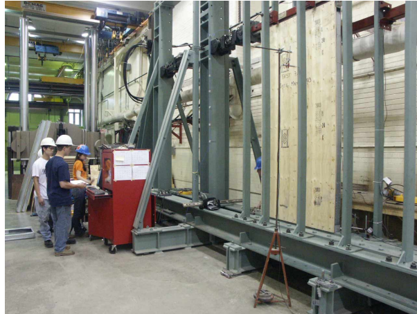
Figure 1: Test frame with 4' x 8' (1220 × 2440 mm) wall specimen
