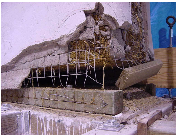
(e) Fracture of mesh and failure of staples at base of Wall E (7.5% drift)
