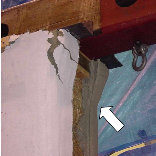
(a) Slip of the box beam at the top of Wall A
