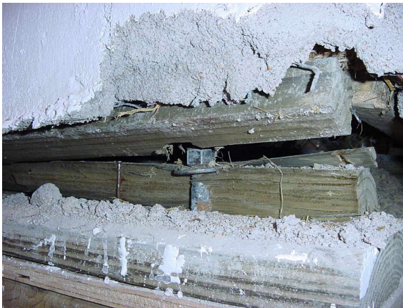
(c) Cross grain tension failure of 2 x 4 sill at base of Wall D (5% drift)
