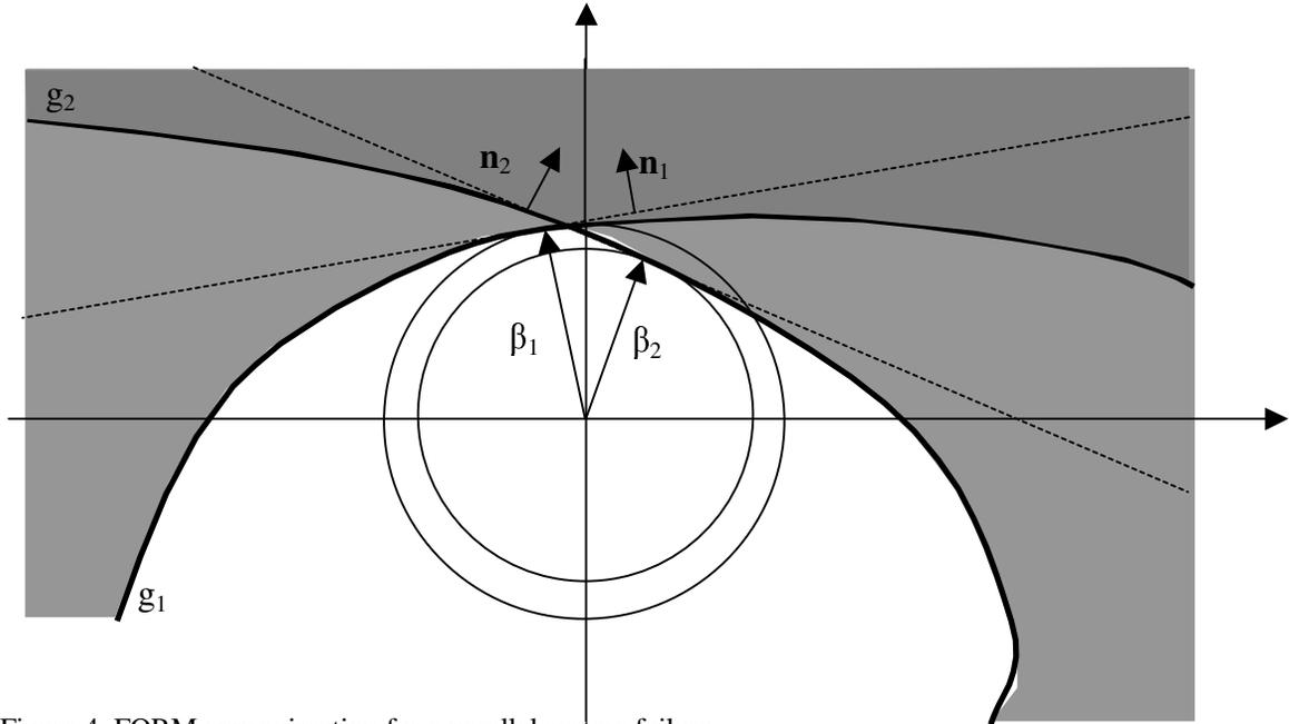
Figure 4. FORM approximation for a parallel system failure.
