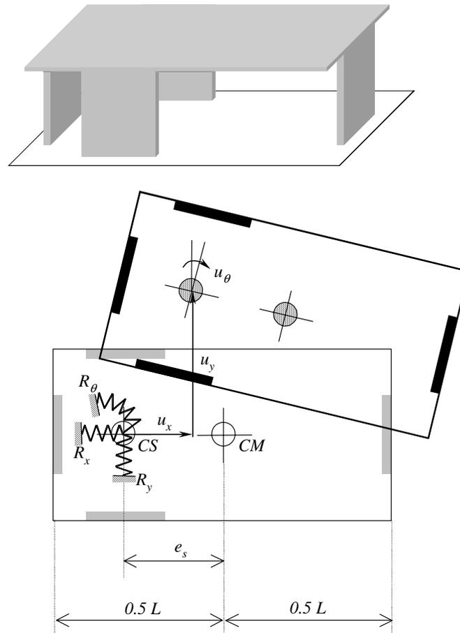
Figure 1. Simplified model of planar asymmetric one-storey building: a rigid deck with three DOF.
