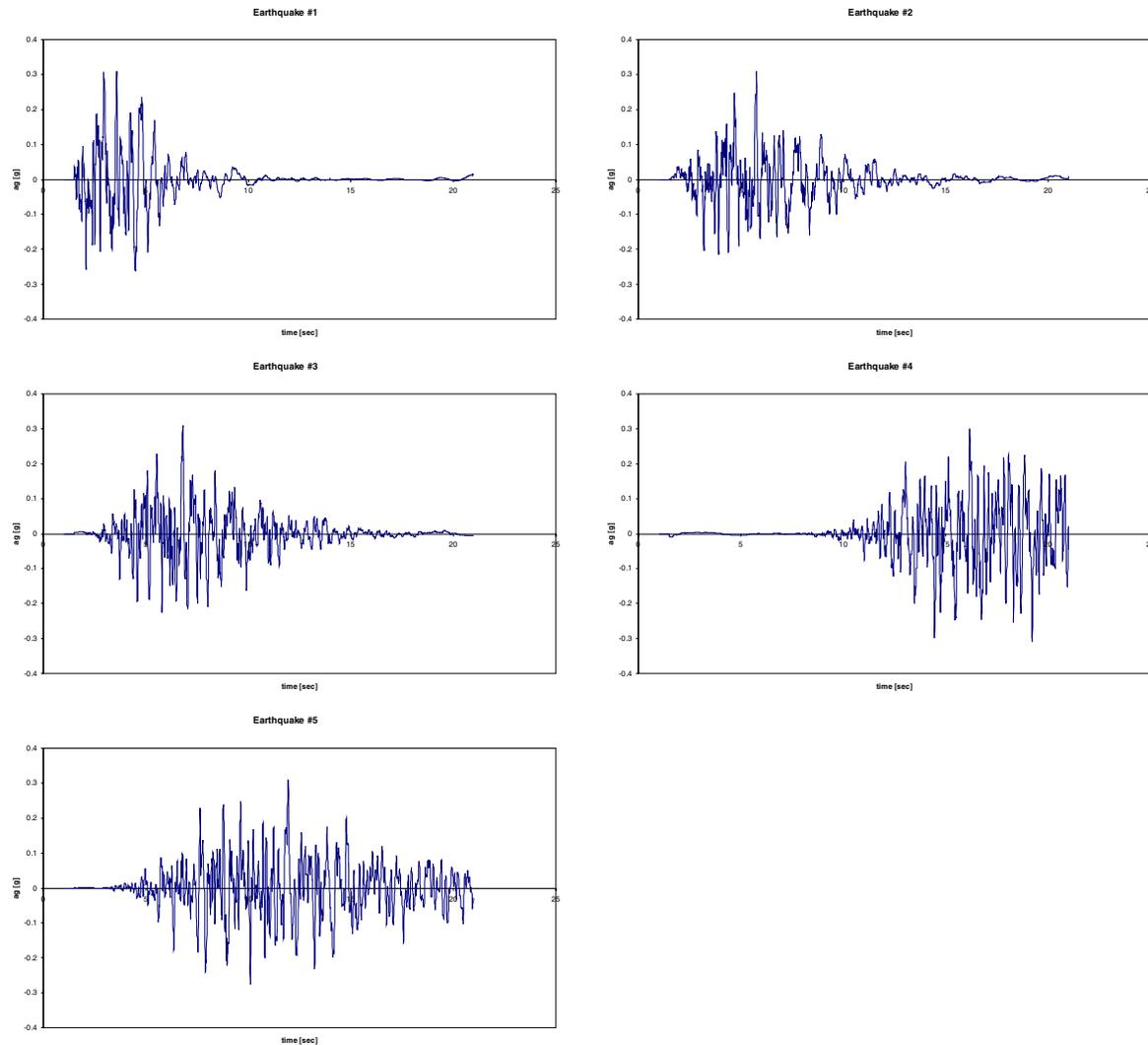
Figure 5. Records used for the dynamic analysis.
