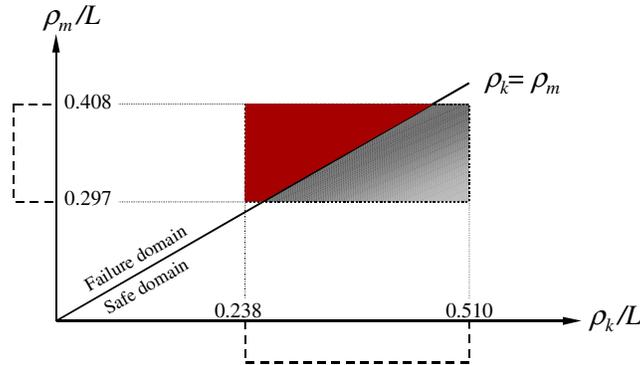
Figure 3. Probability computations according to the second EC8 regularity check. Irregular behaviour is denoted, in standard reliability language, as failure.
