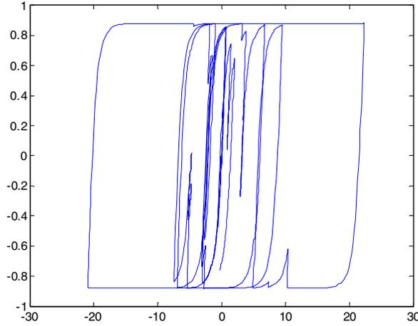
Figure 2. Force-displacement plot for a Bouc-Wen model with  $K_o=110$ ,  $\alpha=0.25$ ,  $A=1$ ,  $\beta=0.8$ ,  $\gamma=0.34$ ,  $n=1$  and  $\delta=0$
