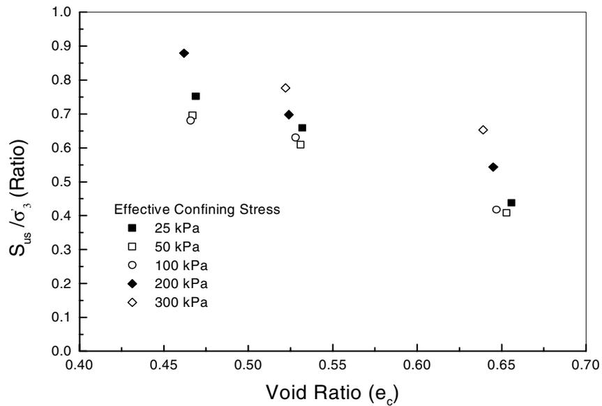
Fig. 19 Variation of normalized residual strength with void ratio
