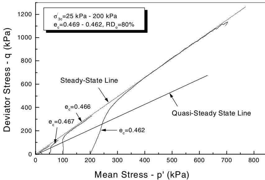
Fig.17 Stress path diagram
