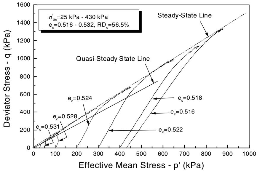
Fig.14 Stress path diagram
