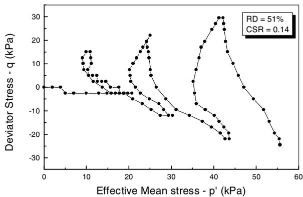
Fig. 8 Variation of mean stress with Deviator stress for Bhuj sample
