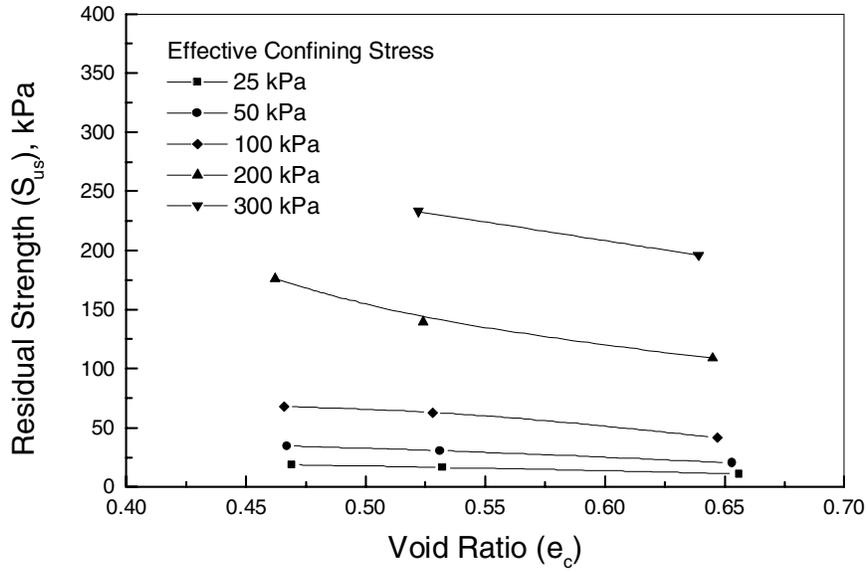
Fig.18 Variation of residual strength with void ratio and confining stress
