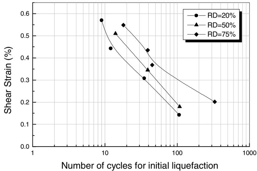
Fig.7 Liquefaction resistance curves for soil samples from Beltaghat
