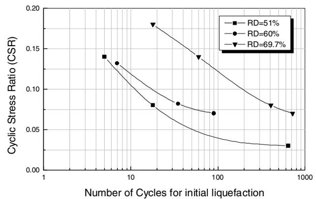
Fig.9 Liquefaction resistance curves for soil samples from Bhuj
