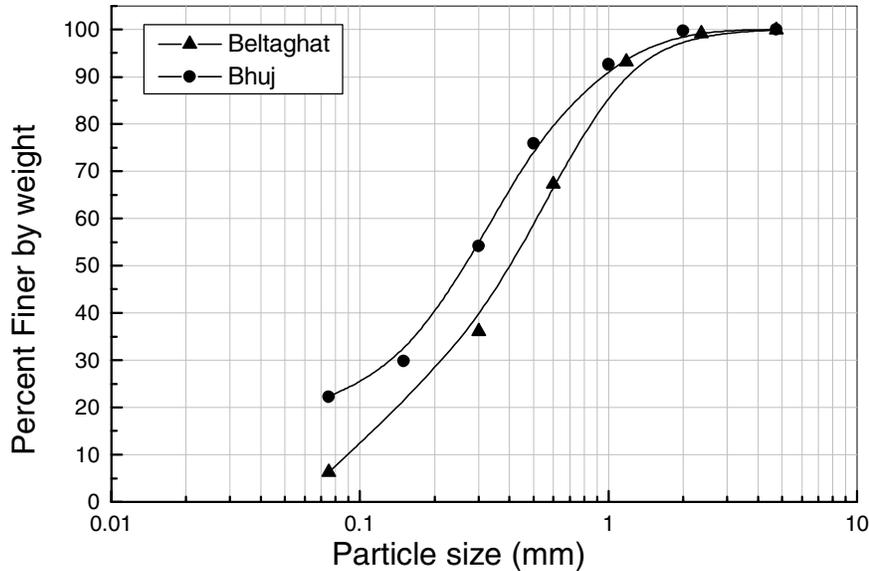
Fig. 5 Grain size distribution of liquefied soils from Beltaghat and Bhuj sites
