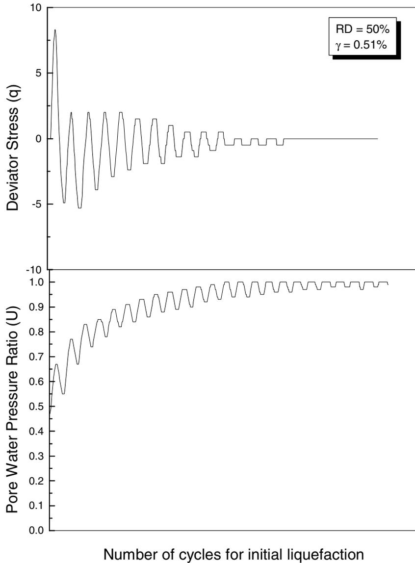
Fig.6 Variation of deviator stress and pore pressure ratio with number of cyclic shear strain
