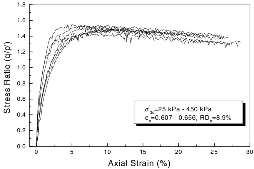
Fig.12 variation of stress ratio with axial strain
