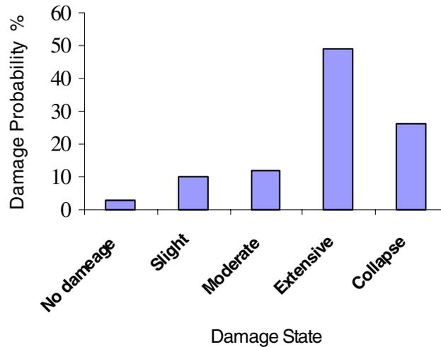
**Figure 2- Damage probabilities vs damage states for bridge category *I*, assuming a PGA value of 0.6g at bridge site (based on Hazus-97 [10])**
