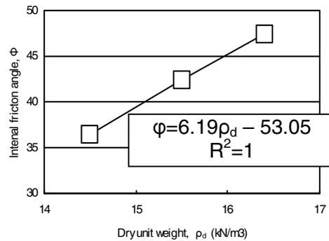
**Figure 5 Relationship between dry weight and internal friction angle****Table 5 Results of plane loading test**
