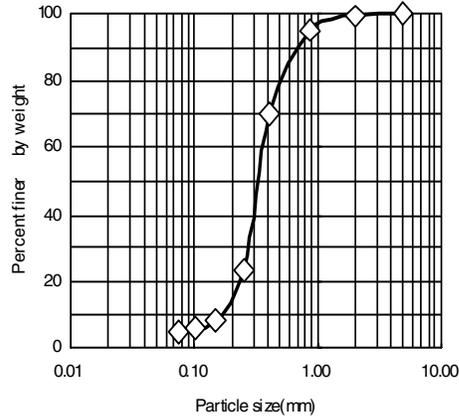
**Figure 2 Grain size distribution of Chiba Sand**
