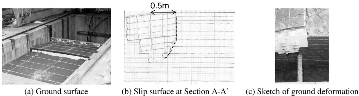
(a) Ground surface (b) Slip surface at Section A-A' (c) Sketch of ground deformation
