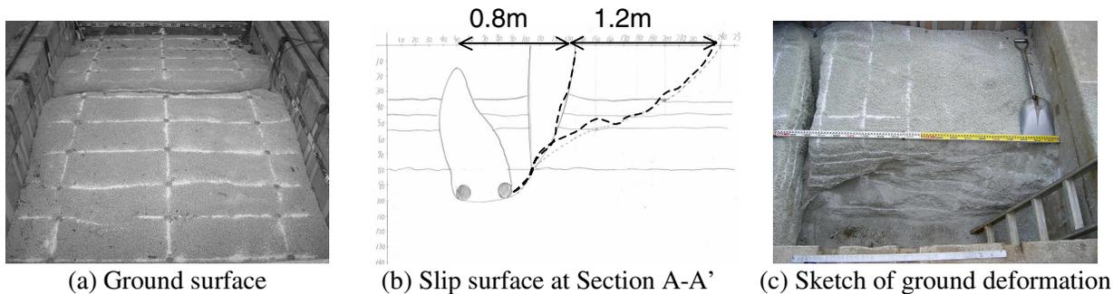
(a) Ground surface (b) Slip surface at Section A-A' (c) Sketch of ground deformation
