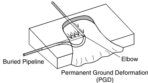
**Figure 10 Assumed phenomenon of a buried pipeline with an elbow subjected to PGD**
