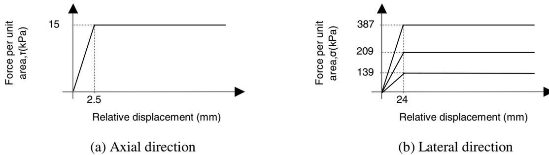
**Figure 12 Soil-pipeline interaction [5, 6, 11]**
