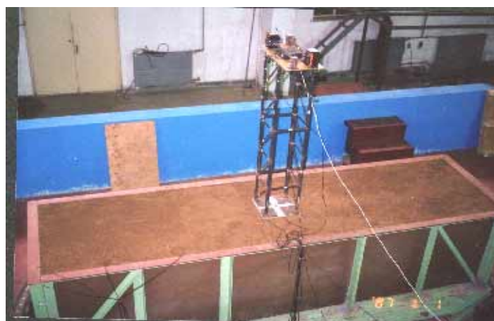
Fig.5 Soil-pile-structure interactive system
