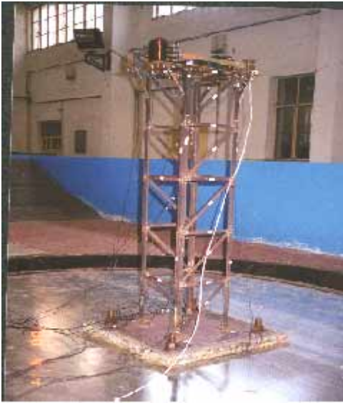
Fig.1 Steel frame structure and TMD device
