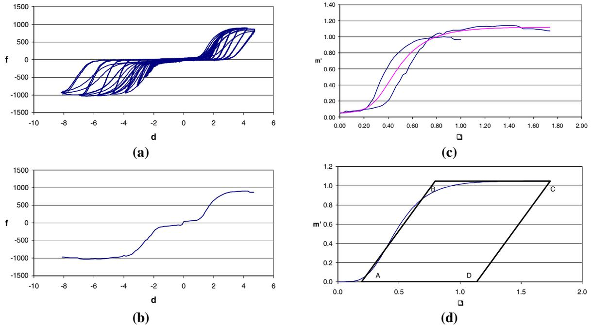
**Figure 8: Sample pipe connector test and analysis results; (a) load-deformation of a “groove”-type joint; (b) enveloping backbone curve; (c) analytical fit of the load deflection curves in the positive quadrant; (d) identified, normalized hysteresis loop.**
