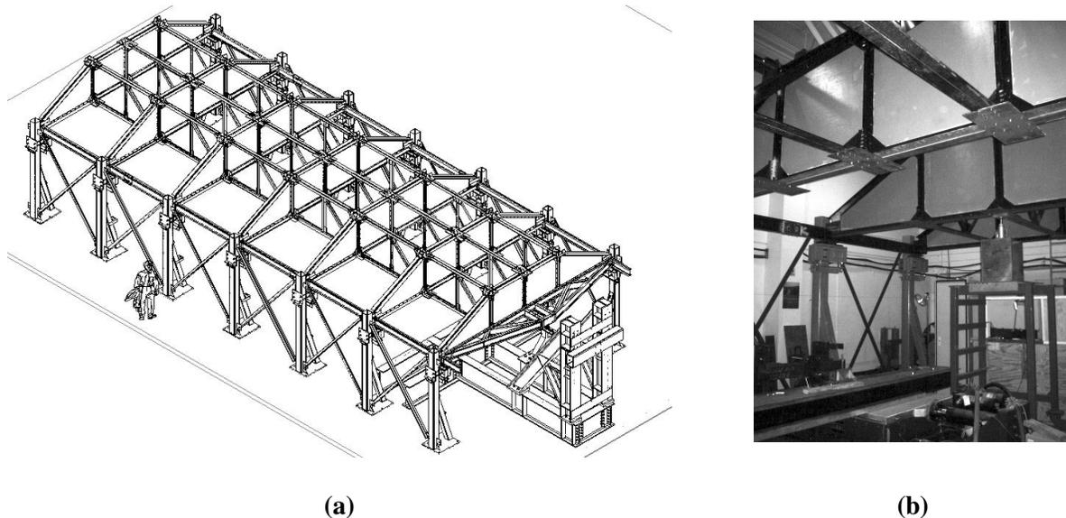
**Figure 9: (a) Solid model of the ceiling test apparatus (notice scale of human operator); (b) a photograph of assembled trusses.**
