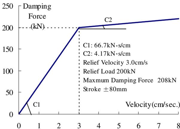
Fig.5. Properties of Design Characteristic of Oil Damper
