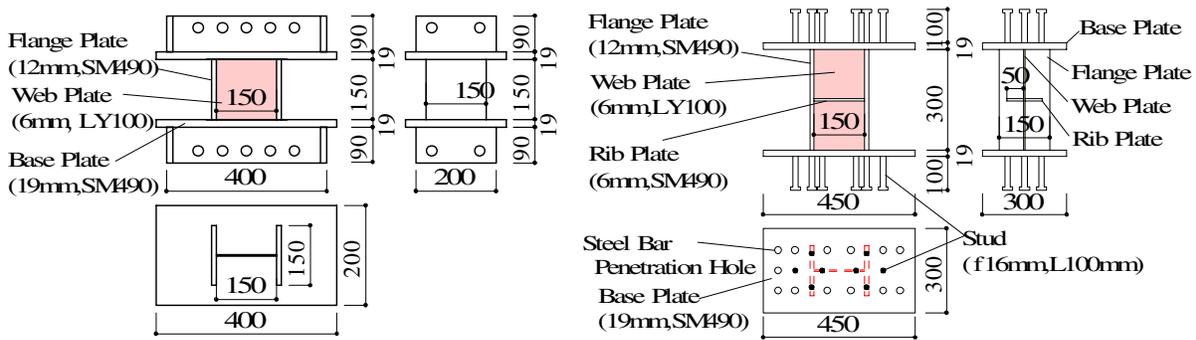
(a) Control-Panel in Control-Column Test      (b) Control-Panel in Control-Column and Control-Brace Test
