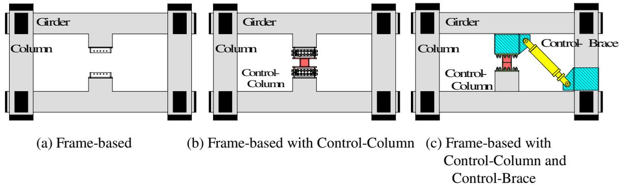
Fig.2. RC Frame Models
