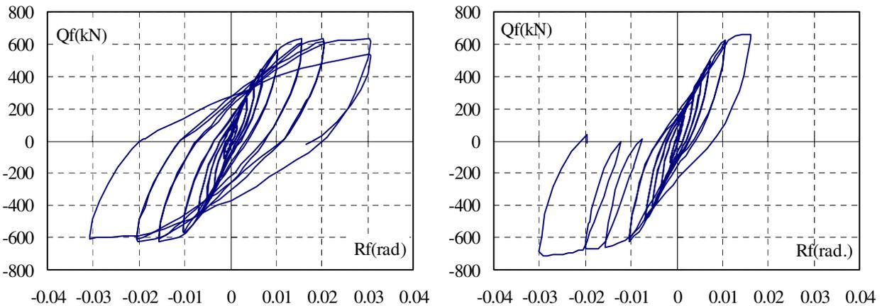
(a) Control-Column Test (b) Control-Column and Unbonded Brace Test
