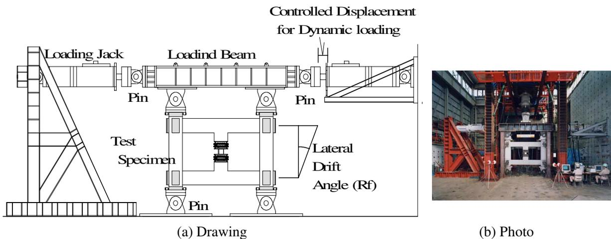
Fig.7. Test Setup
