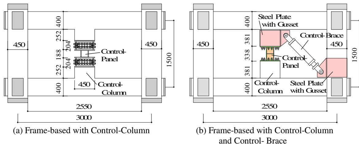
Fig.3. Test Specimens
