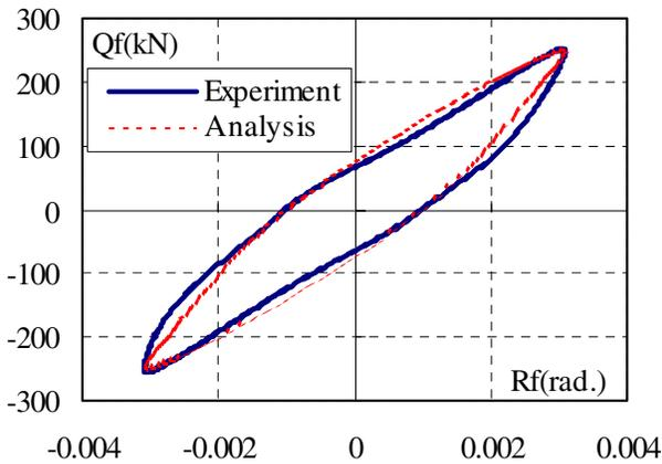
(a) Control-Column and Oil-Damper Brace in Dynamic Loading
