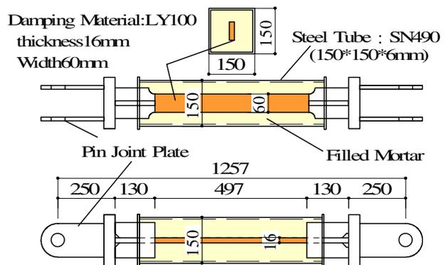
Fig.6. Unbonded Brace
