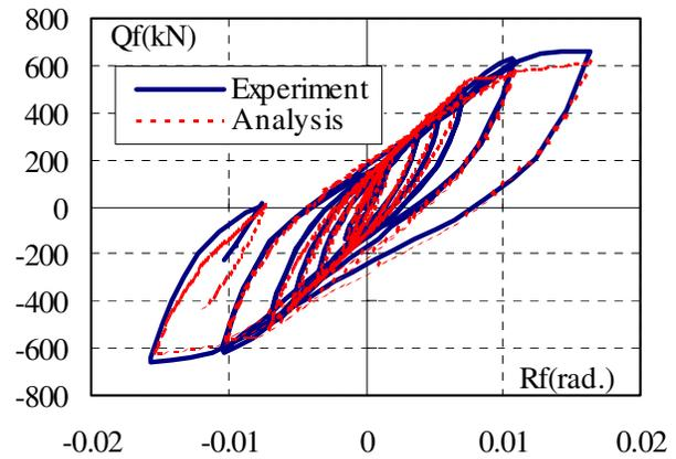
(b) Control-Column and Unbonded Brace in Static Loading
