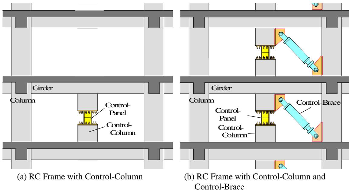
Fig.1. RC Frame with Energy Dissipation Devices
