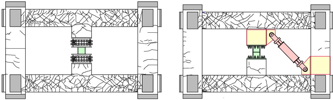
(a) Control-Column Test (b) Control-Column and Control-Brace Test
