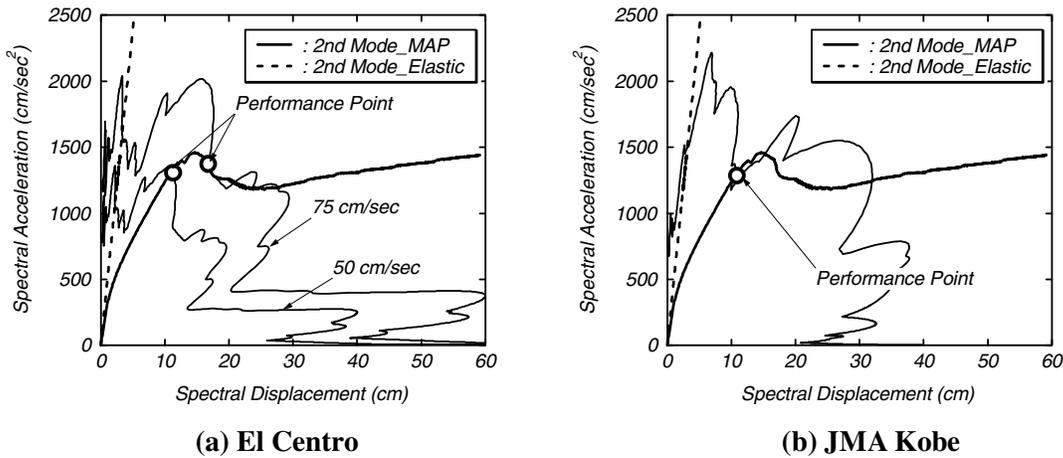
**Fig. 8 Relation between Capacity Spectrum for the 2nd Mode and Demand Spectrum**
