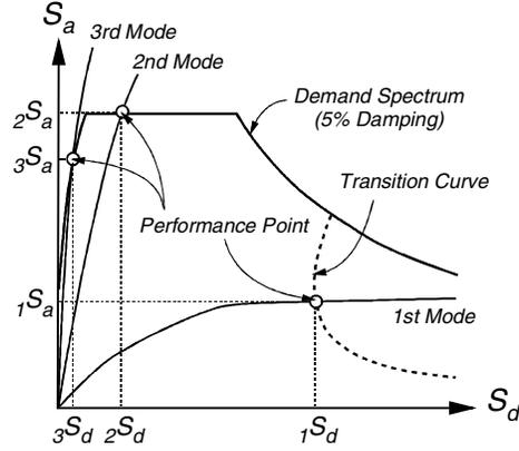
**Fig. 5 Illustration of Modal Capacity Spectrum Method**
