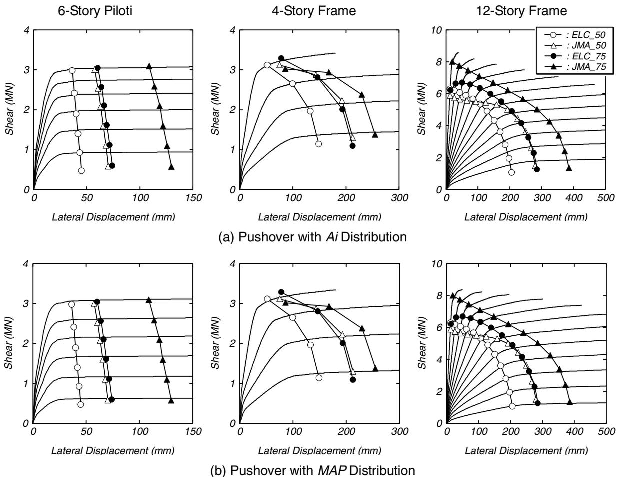
**Fig. 2 Story Shear versus Lateral Displacement Relationships**
