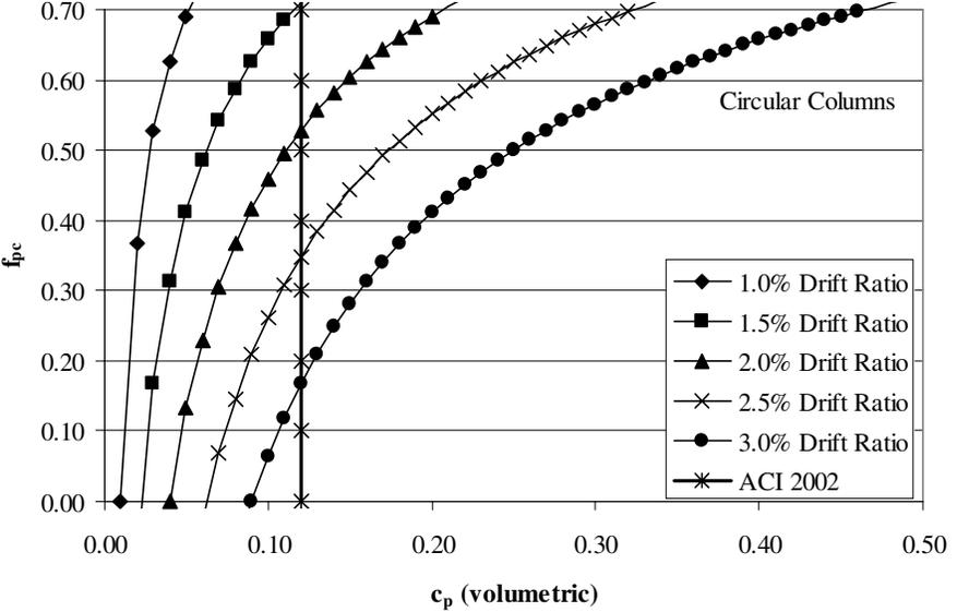
Fig. 8. Interaction between  $c_p$  and  $f_{pc}$  for circular columns with various limiting drift ratios.
