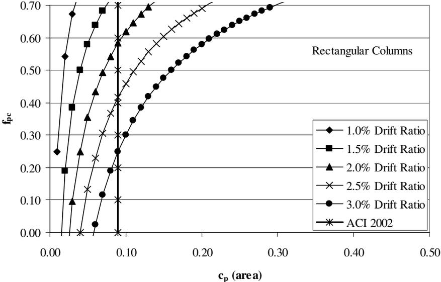
Fig. 7. Interaction between  $c_p$  and  $f_{cp}$  for rectangular columns with various limiting drift ratios
