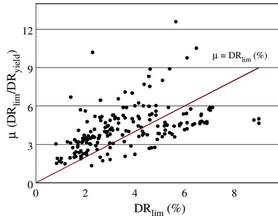
Fig. 2. Ductility ratio versus limiting drift ratio
