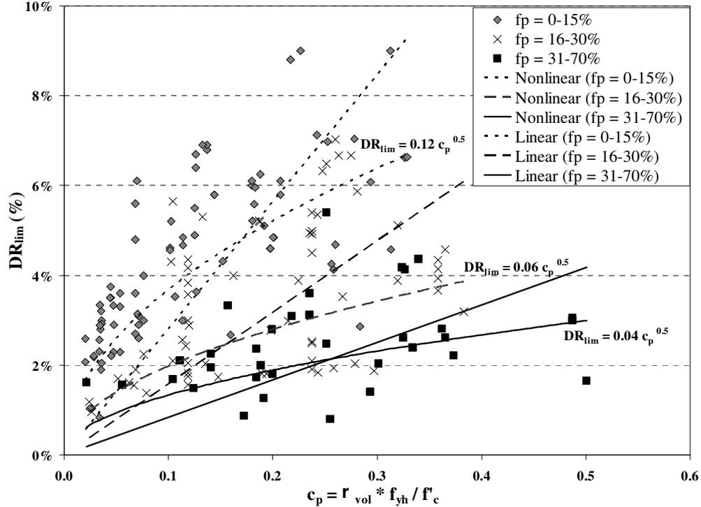
Fig. 3. Limiting drift ratio versus volumetric confinement parameter
