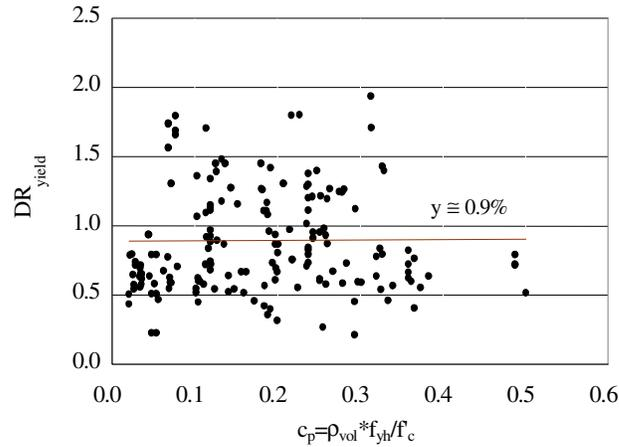
Fig. 1. Drift ratio at yield versus volumetric confinement parameter
