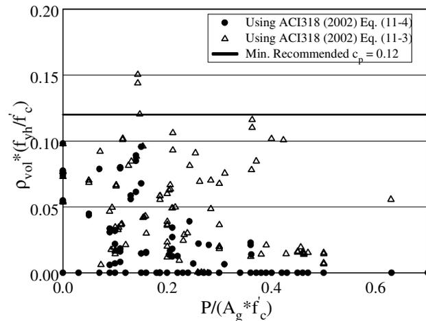
Fig. 6. Required volumetric  $c_p$  for developing  $M_y$  versus  $f_p$ ,  $V_c$  calculated using Eq. (10) and (11)
