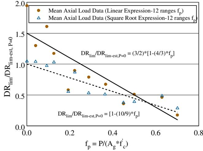
Fig. 4. Ratio of  $DR_{lim}/DR_{lim,est}$  for  $P=0$  vs. mean axial load ratios
