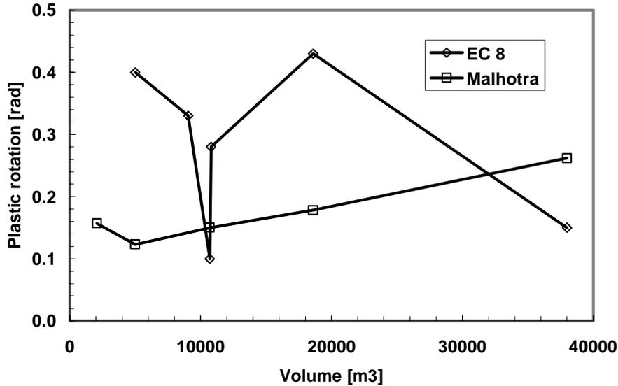
**Figure 7. Plastic rotation versus fluid volume.**
