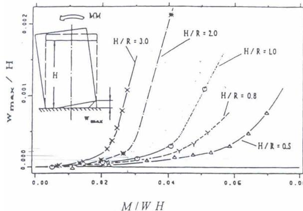
**Figure 1: Maximum uplift height versus overturning moment  $M/WH$  ( $M$ : moment;  $W$ : total liquid weight;  $H$ : liquid height); Figure A11 of EC8, part 4.**
