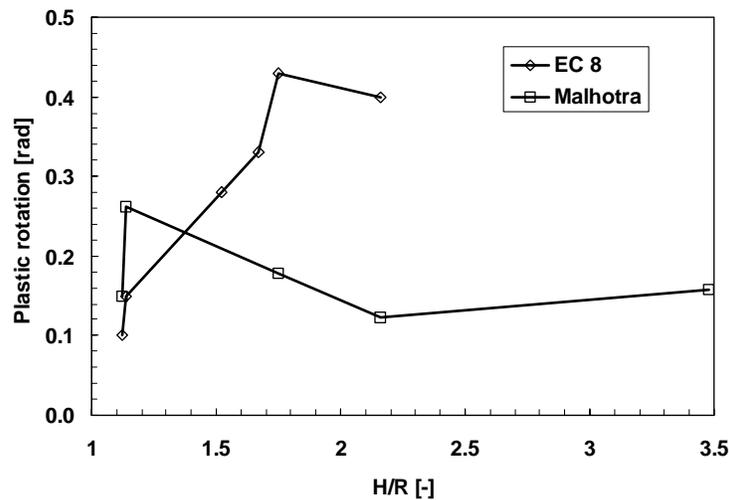
**Figure 6. Plastic rotation versus  $H/R$ ; the result for the tank with  $H/R = 3.48$  (“Vernier”) would be far above the uppermost value (0.5) of the graph.**
