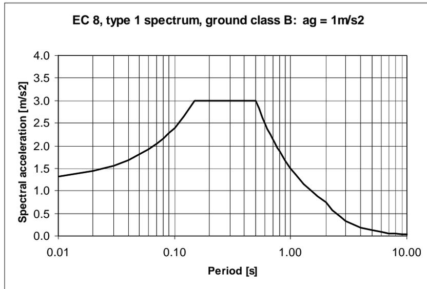
**Figure 5. Acceleration response spectrum used for the seismic calculation of tanks.**
