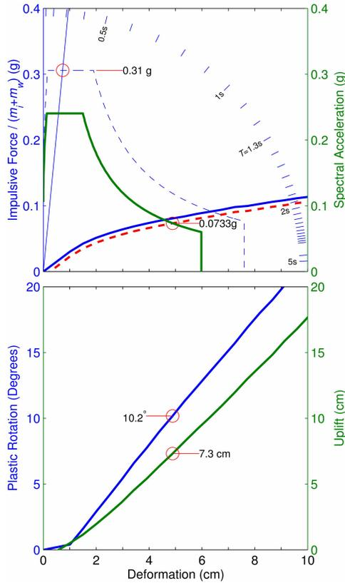
**Figure 3. Static pushover analysis from skeleton stiffness and response spectrum (top). Plastic rotation and base uplift (bottom).**
