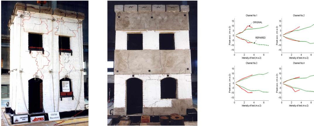
**Figure 9. Two storey brick masonry model after seismic tests: original and repaired**
