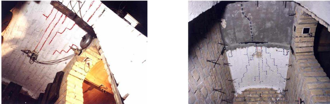
**Figure 10. Cracks in the vault after the tests of two storey masonry model: original – on the left; repaired with fibre plaster – on the right**
