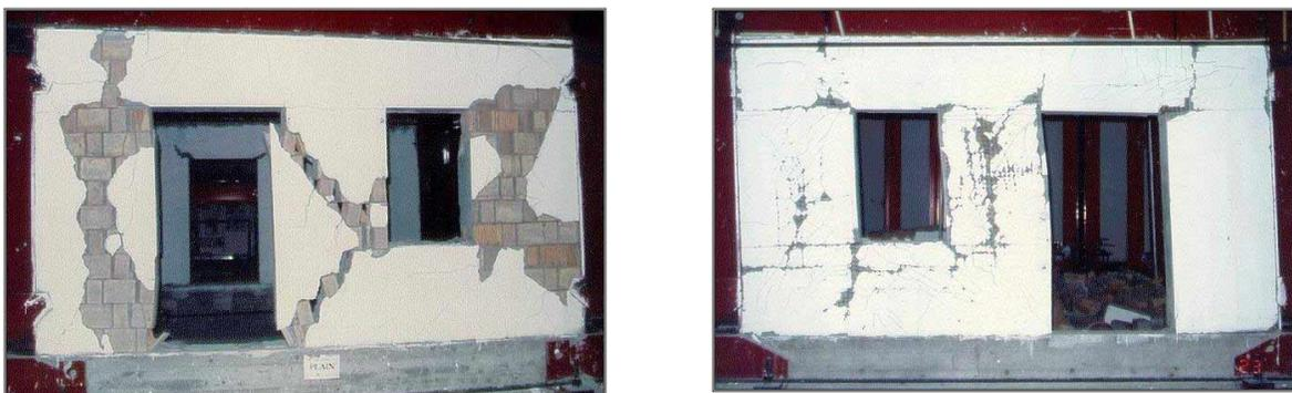
**Figure 11. Cracks in the masonry wall after pseudodynamic tests of wall with openings: original – on the left; repaired with polymer grids in plaster – on the right**
