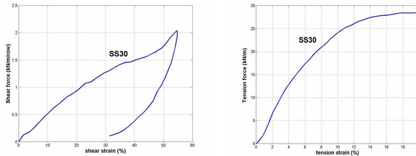
**Figure 8. Behaviour of polymer grids in shear and tension obtained on small samples**
