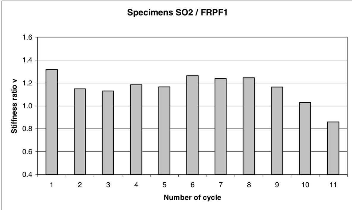
**Fig. 5 Stiffness comparison between strengthened specimens SO<sub>2</sub> and FRPF<sub>1</sub>**
