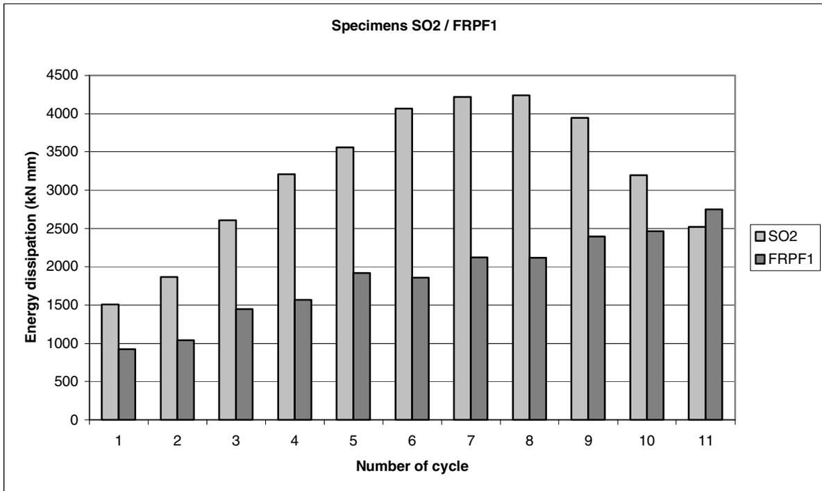
**Fig. 6 Energy dissipation comparison between strengthened specimens SO<sub>2</sub> and FRPF<sub>1</sub>**
