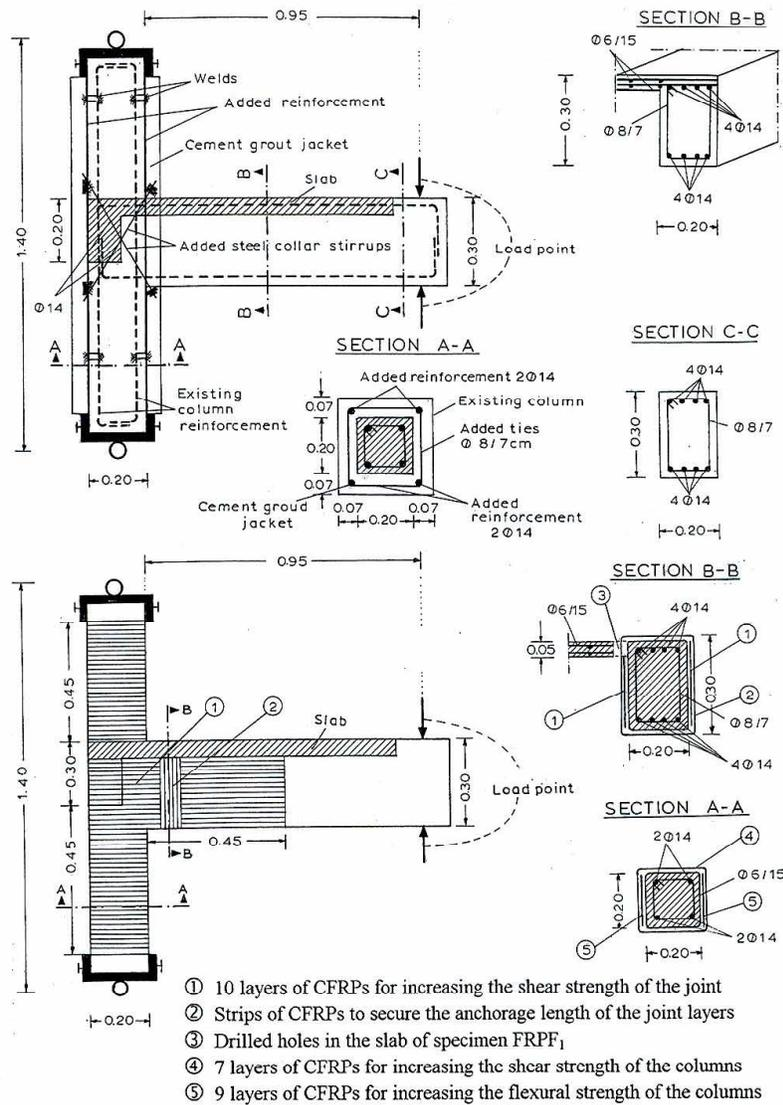
**Fig. 2 Jacketing of column and beam-column connection of subassemblages SO<sub>2</sub>, SP<sub>2</sub>, FRPF<sub>1</sub> and FRPS<sub>1</sub> (dimensions in m)**
