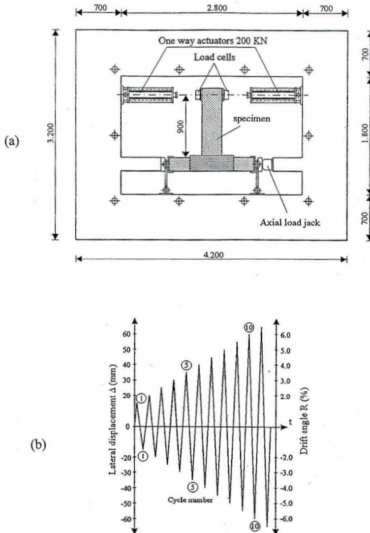
Fig. 3 (a) Test setup (dimensions in mm), (b) Lateral displacement history
