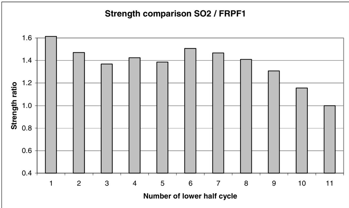
**Fig. 7 Strength ratio of specimen SO<sub>2</sub>, to specimen FRPF<sub>1</sub>**
