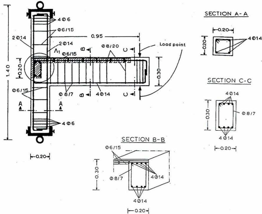
**Fig. 1 Dimensions and cross-sectional details of original specimens F<sub>1</sub>, S<sub>1</sub>, O<sub>2</sub> and P<sub>2</sub> (dimensions in m)**
