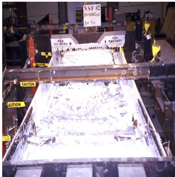
Crushing of Concrete Wall
