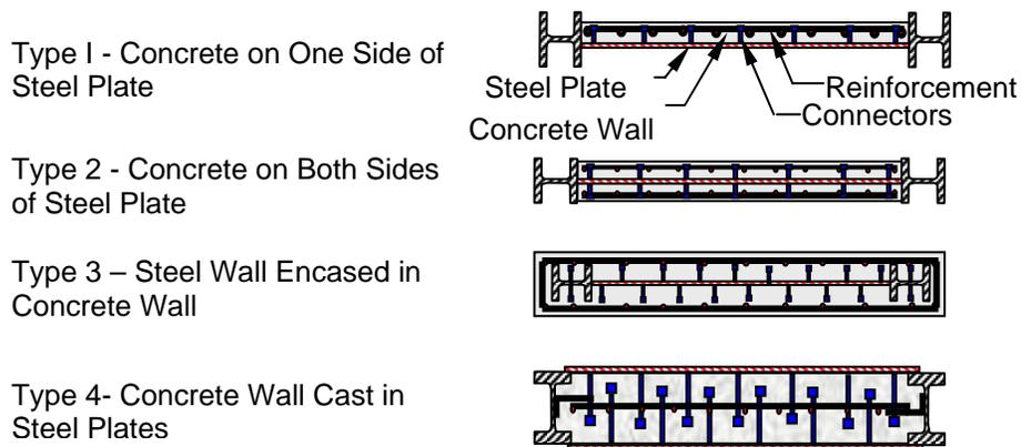
**Figure 1. Composite Shear Wall Systems (Astaneh [6])**
