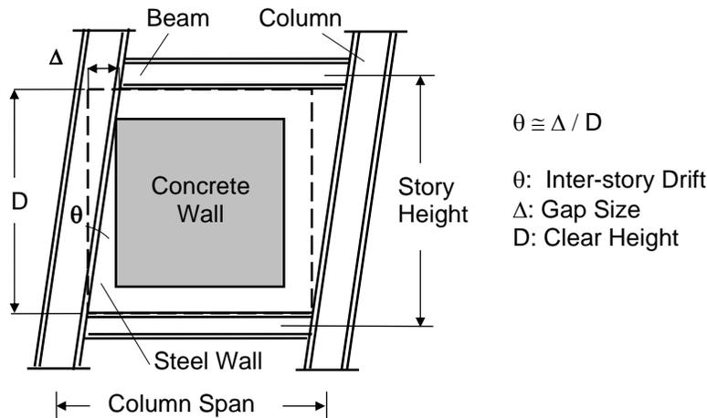
**Figure 3. Function of Gap in the Innovative Composite Shear Wall System**
