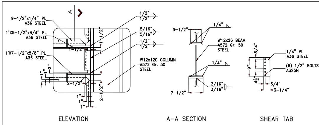
**Figure 6. Beam to Column Moment Connections**
