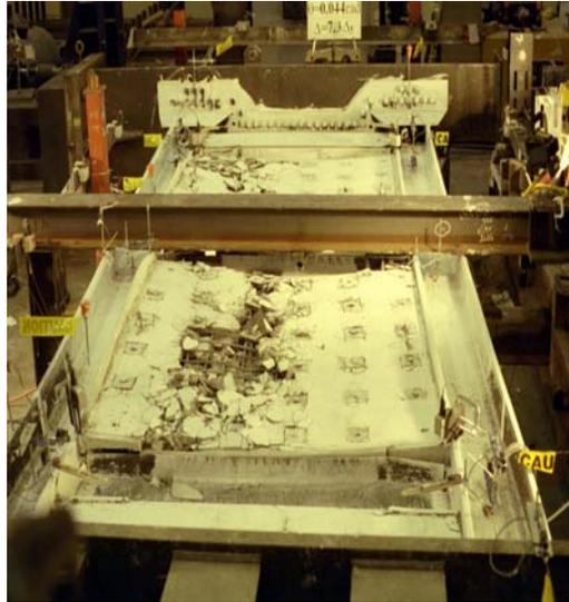
Crushing of Concrete Wall
