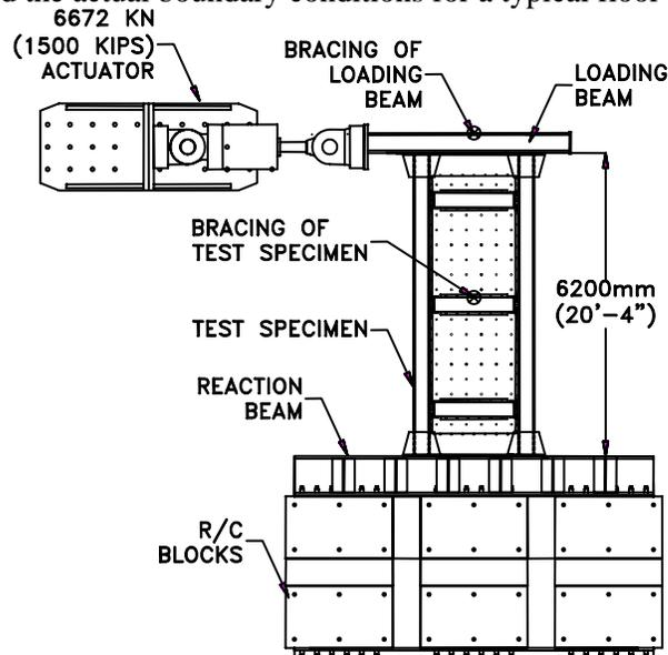
**Figure 7. Test Specimen and Test Set-up**
