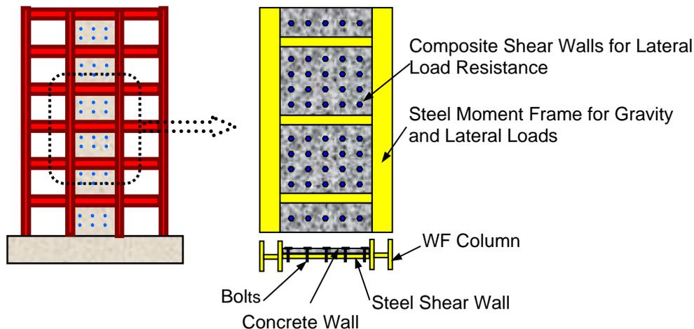
**Figure 4. Generic Structures and Test Specimen**
