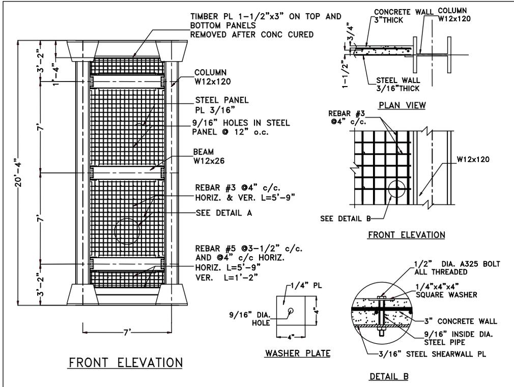
**Figure 5. A Specimen with Details of Concrete Shear Wall**
