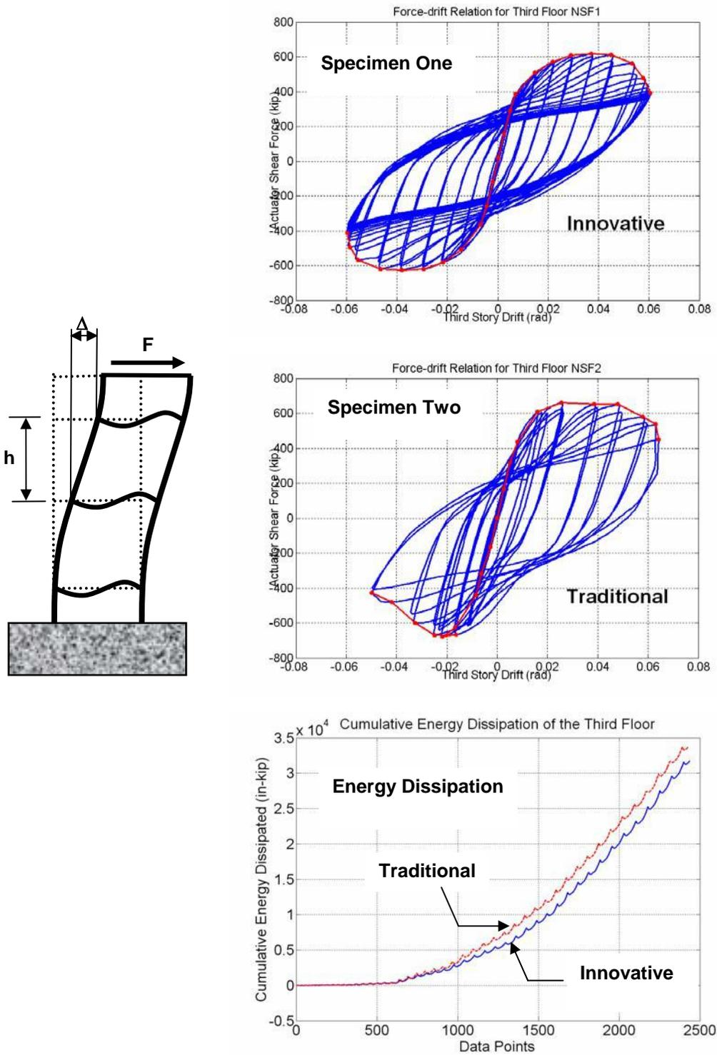
Figure 11. Shear Force- Displacement and Energy Dissipation Curves for Third Floor
