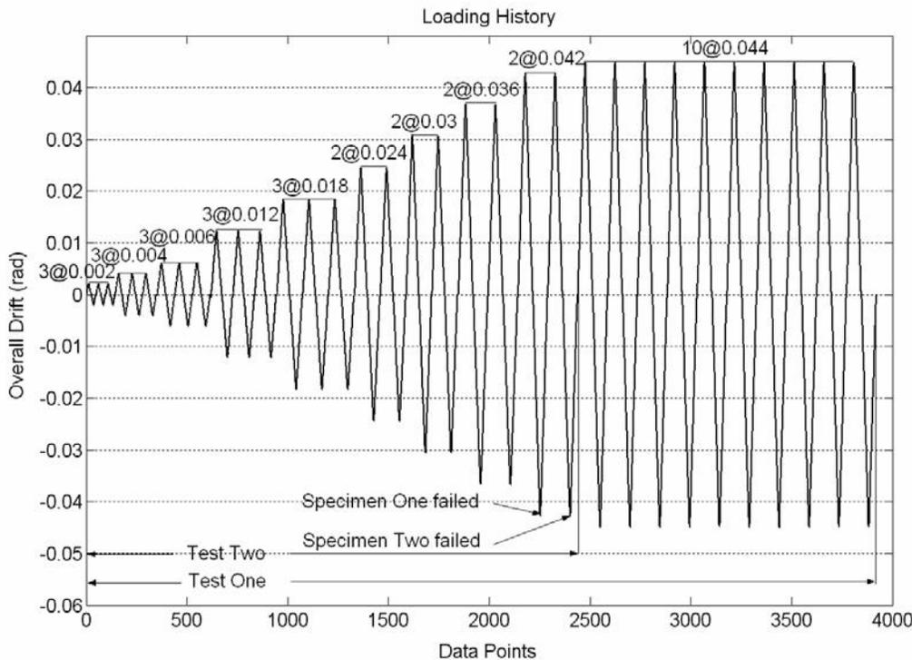
**Figure 8. Loading History Applied to Both Specimens**
