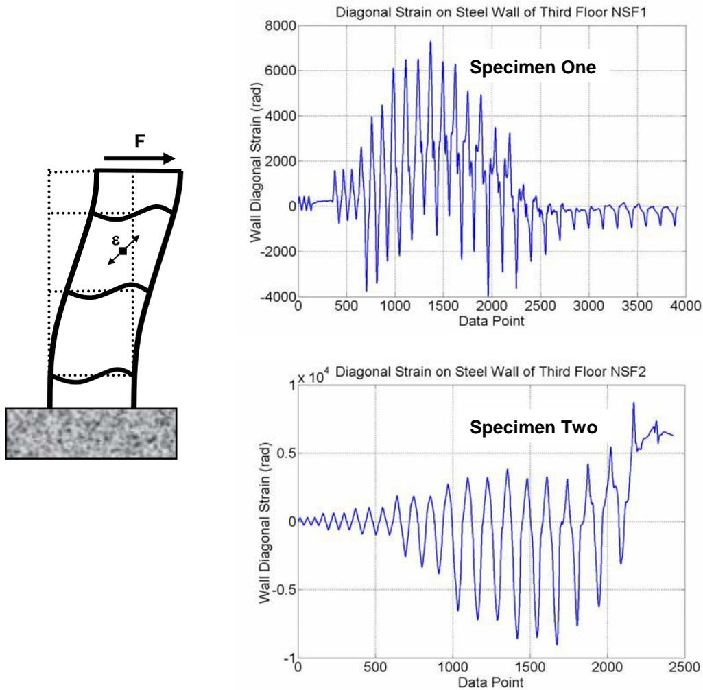
**Figure 12. Diagonal Strain on Third Floor of Two Specimens**
