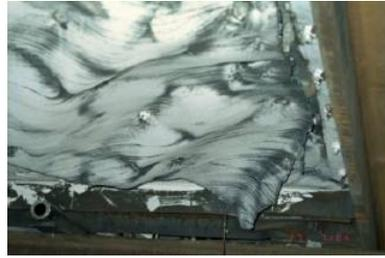
Fracture of Steel wall
