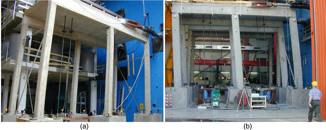
Fig. 15. View of the prototypes during the pseudodynamic tests: (a) cast-in-situ and (b) precast frame.
