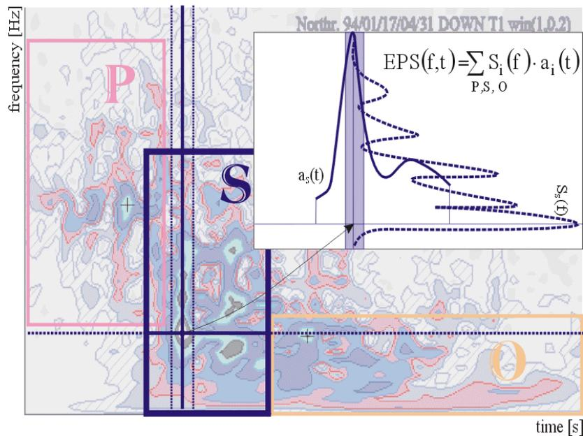
**Fig. 4 Approximating load of evolutionary sub-processes corresponding to distinct wave fields P, S (pronounced) and C/G or O by a product of slices representing spectral and temporal modulation, crossing at the maximum peak of the wave phases, used for parametric shape functions fitting**
