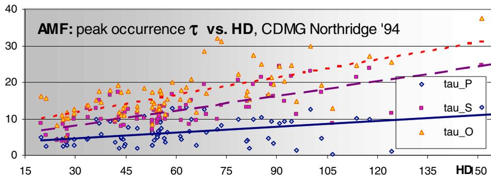
**Fig. 12 Peak occurrence  $\tau$  of AMF (5) vs. hypo-central distance for the dataset of N94 and the three wave phases of the load model (1)**
