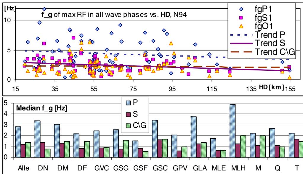
**Fig. 8** Distribution of the strongest resonance frequency in the P,S and O=C\G wave phases of the estimated load model versus hypocentral distance (upper) und for site classes (lower part), CDMG, N94. Site classes are with respect to distance (D\* for near, middle and far field), regional adjacency, i.e., close range of azimuth (G\*) and soil classes according to Park 1998 [16].
