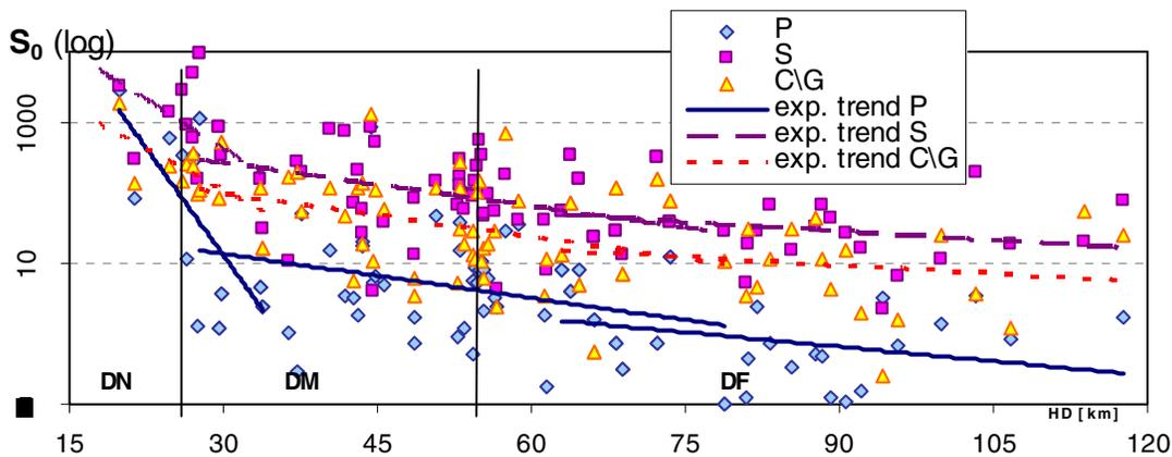
**Fig. 10** Incitation  $S_0$  corresponding to the strongest resonance frequency of the modeled wave phases versus hypo-central distance, exp. trends separately for near, middle and far field records, N94
