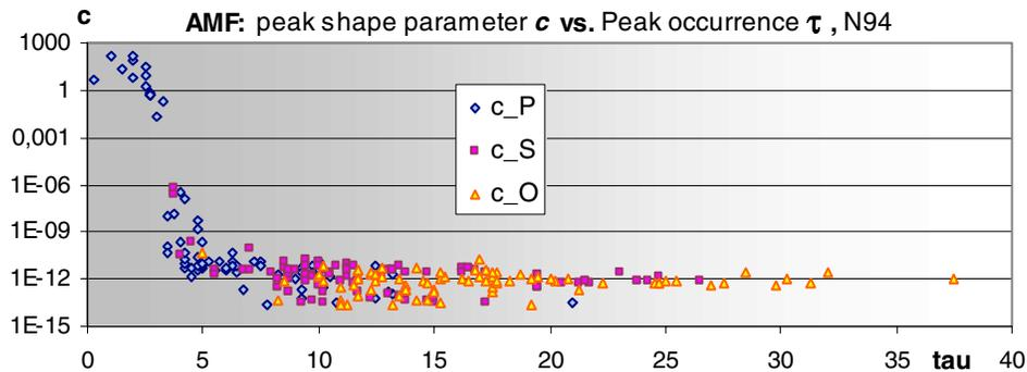
**Fig. 11 Peak shape parameter  $c$  of AMF (5) versus peak occurrence  $\tau$  of the modeled wave phases, N94 dataset. In the P wave phase (diamonds), LSQ fits to approximations were realistic and hence results for  $c_P$  are reliable, showing a clear connection between both parameters.**
