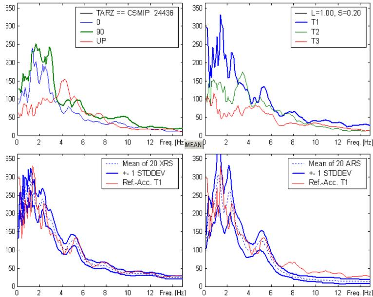
**Fig. 13** Velocity response spectra with 5% damping of the original components and components transformed onto time-dependent stochastic principal axes (upper left and right), Average vel. response spectrum of a sample of 20 time histories for the intermediate steps of load approximation and least-squares fitting (bottom left and right, resp.), each of the latter re-normalized at the total energy of the evol. spectrum of the reference component T1, N94, TARZ (near field with hill resonance).
