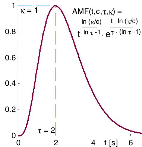
**Fig. 3** Definition and meaning of the parameters of amplitude modulation function (5)
