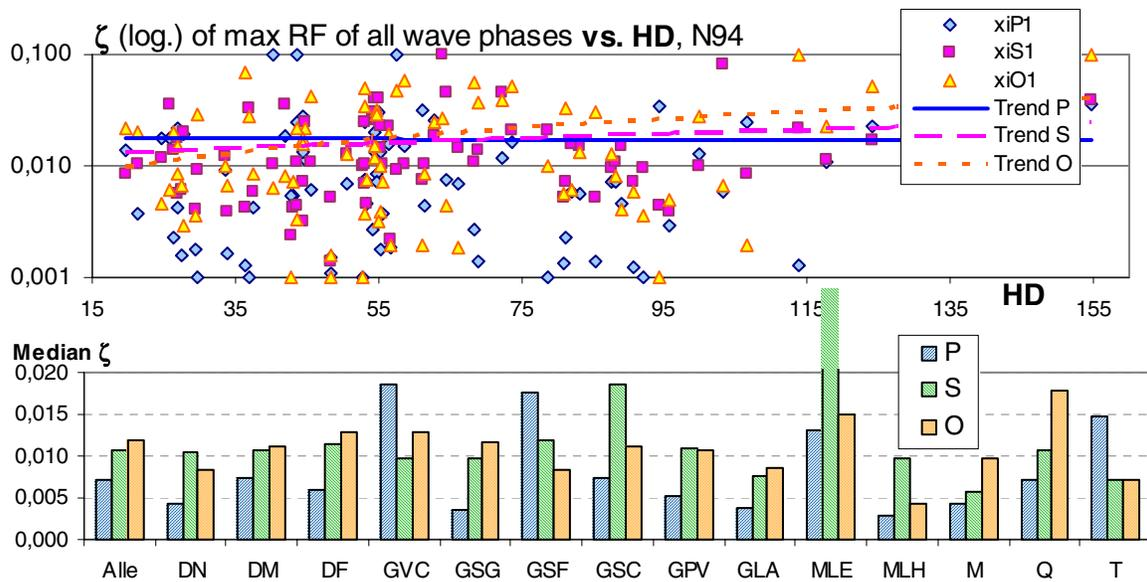
**Fig. 9 Distribution vs. hypocentral distance (upper part) and median analysis for damping parameter  $\zeta$  of the strongest resonance frequency in the estimated models, no significant trends.**
