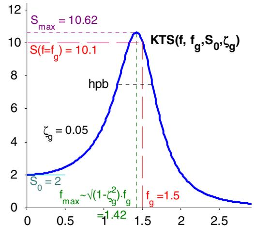
**Fig. 1** shape characteristics and distinctive parameters of the Kanai-Tajimi-Spectrum
