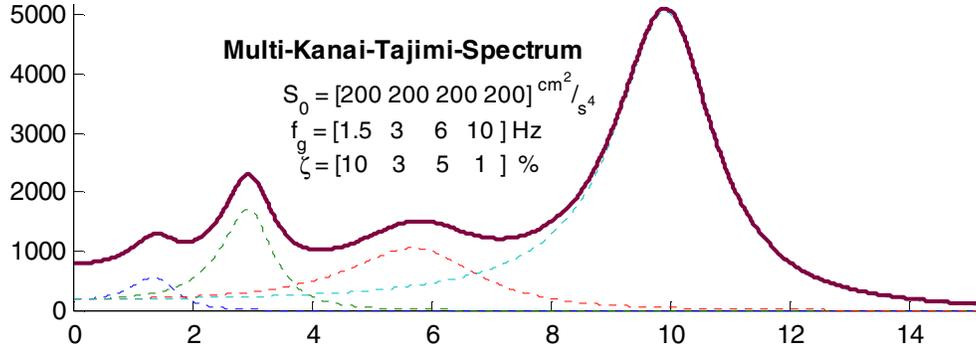
**Fig. 2** Example of a Multi-KTS with four modes of resonance and distinct damping values, caused by an incident wave field of total acc. evolutionary spectral amplitude  $\Sigma S_0 = 800 \text{ cm}^2/\text{s}^4$ .
