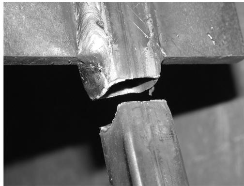
**Figure 8. Typical failure of 20x20x2.0SHS long specimen (Series 3)**
