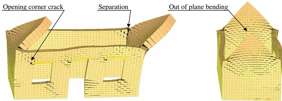
Fig.8 Deformation just before the collapse of the house when earthquake of the maximum acceleration  $300 \text{ cm/sec}^2$  shakes in the right-left direction
