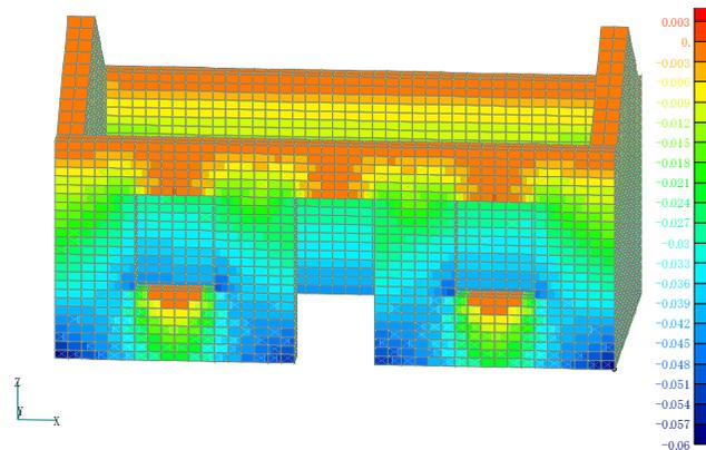
Fig.6 Distribution of the confining stress in the z-x plane (MPa)
