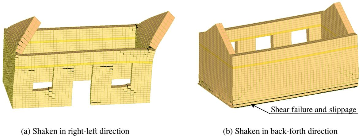
Fig.11 Deformation of the house retrofitted with “Method 1”
