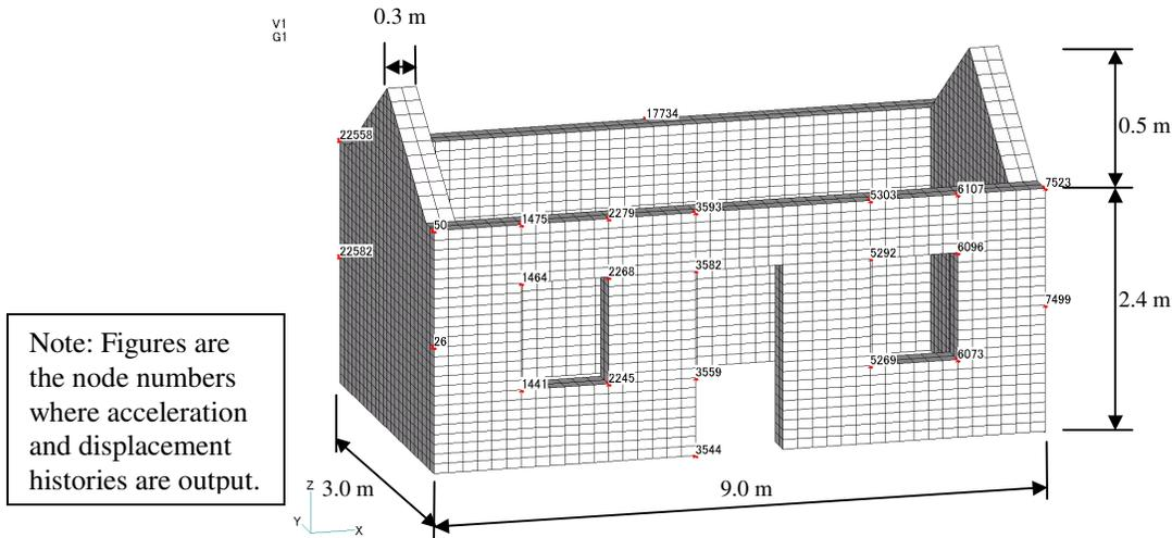
Fig.5 Model used in the analysis
