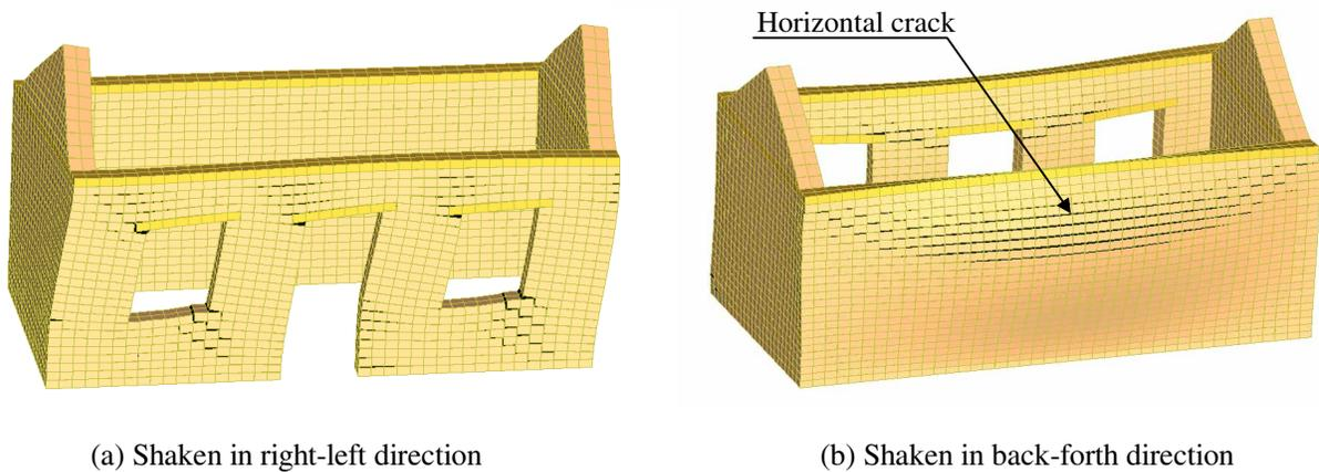
Fig.12 Deformation of the house retrofitted with “Method 2”
