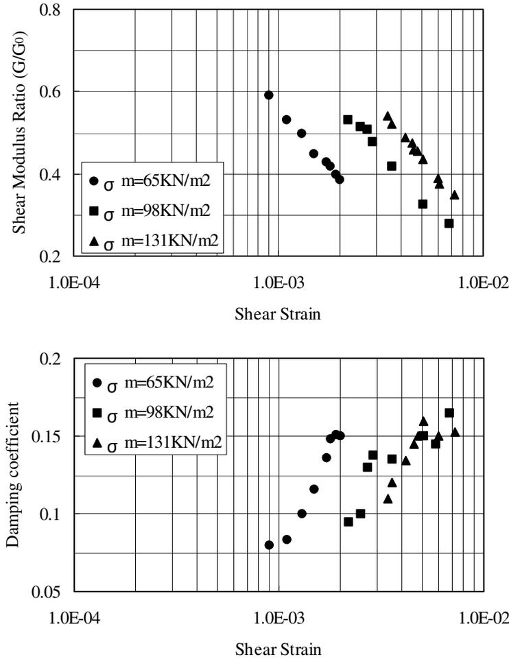
Fig.4 Dependency of shear modulus and damping coefficient on shear strain (Islam and Watanabe [7])
