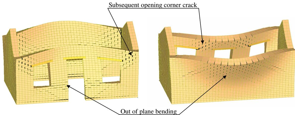
Fig.9 Deformation just before the collapse of the house when earthquake of the maximum acceleration  $300 \text{ cm/sec}^2$  shakes in the back-forth direction
