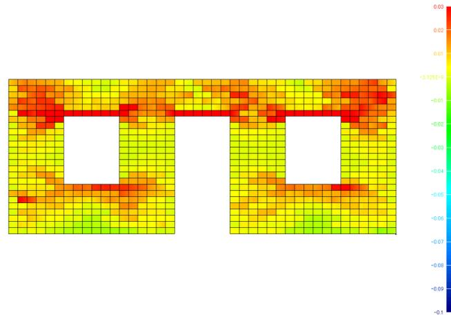
Fig.7 maximum tensile stress distribution (MPa)
