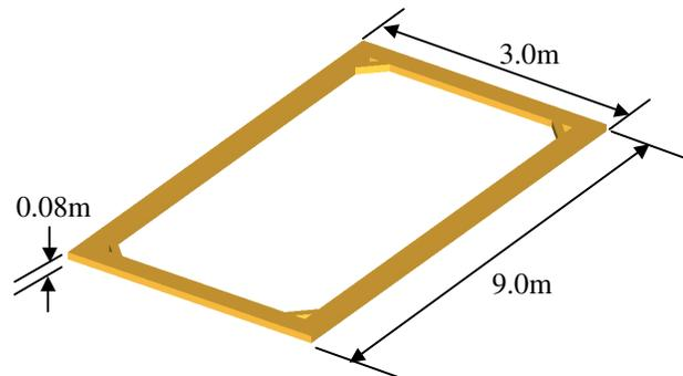
Fig.10 Wooden frame used for retrofitting
