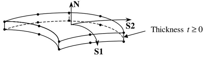
Fig.2 Viscoelastic joint element
