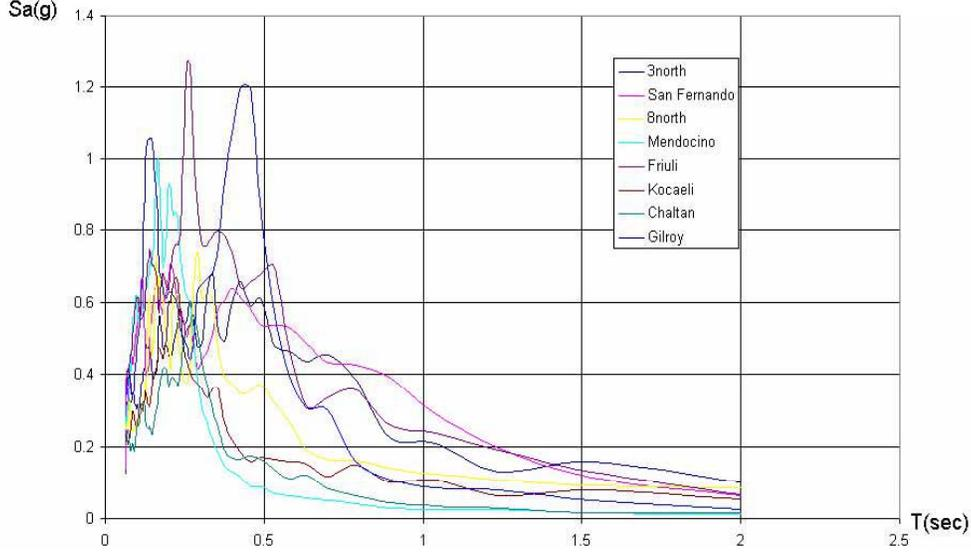
Fig 1. Response Spectra of the eight accelerograms.
