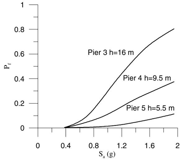
Fig. 3 Fragility curves of three pier of Vallone del Duca via-
