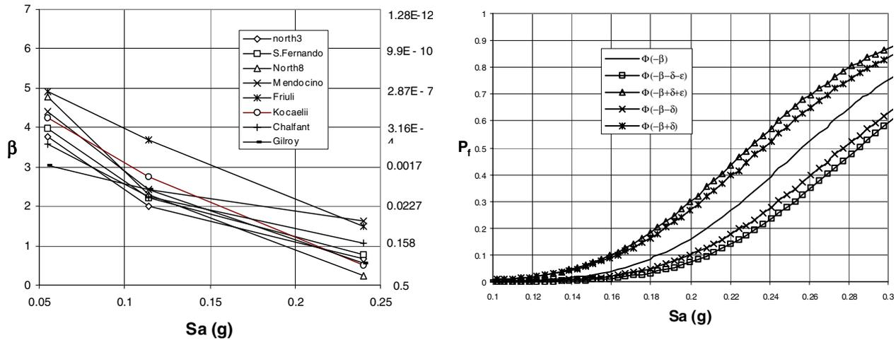
Fig. 5 Olmeta viaduct, pier n. 2: (left) Reliability index  $\beta$  for different accelerograms vs. the spectral acceleration; (right) Fragility curve and sensitivity of error model and variability of response.
