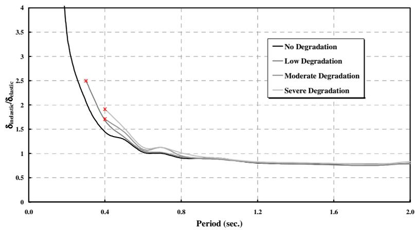
**Figure (8) Displacement Estimates for Clough Model – R=8**
