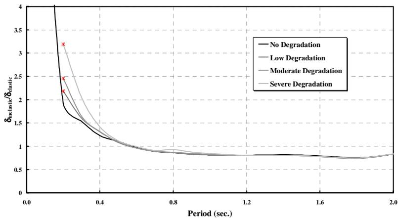
**Figure (5) Displacement Estimates for Clough Model – R=4**
