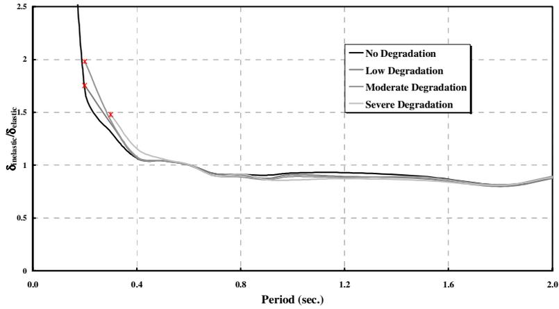
**Figure (4) Displacement Estimates for Bilinear Model – R=4**
