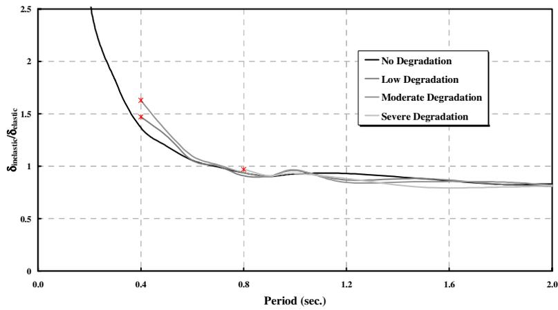
**Figure (7) Displacement Estimates for Bilinear Model – R=8**
