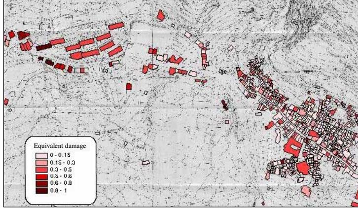
**Figure 8. Equivalent damage map in Castelluccio.**
