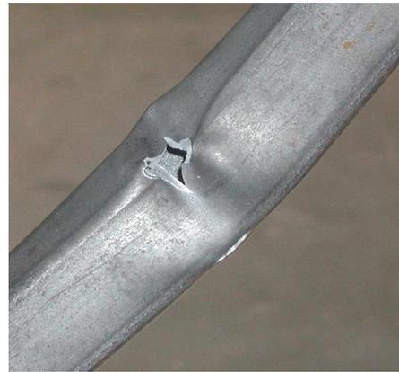
**Figure 7 – Local buckling and partial fracture**
