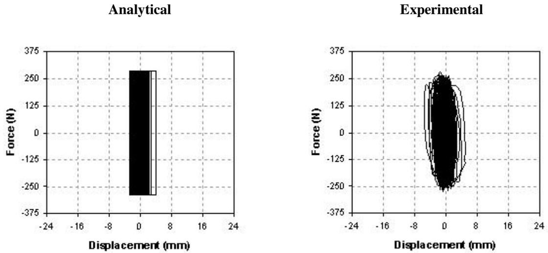
Figure 9. Hystereses for peak table acceleration of 0.27g in X-direction of the piping system
