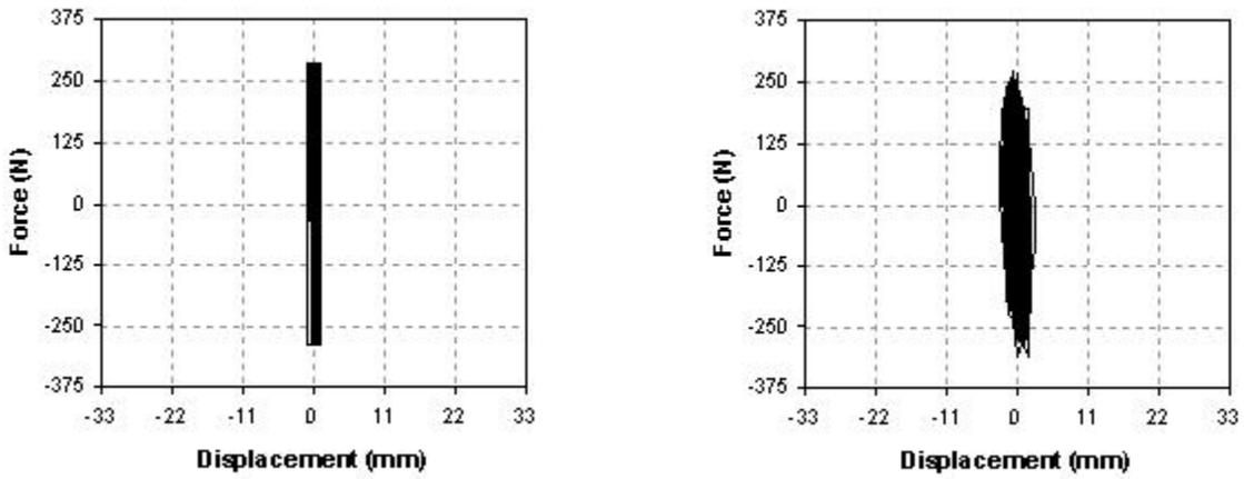
Figure 13. Hystereses for peak table acceleration of 0.22g in Z-direction of the piping system
