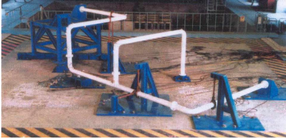
Figure 3. Test setup of the piping system with friction damper
