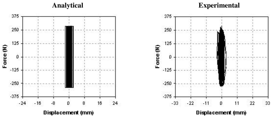
Figure 8. Hystereses for peak table acceleration of 0.2g in X-direction of the piping system
