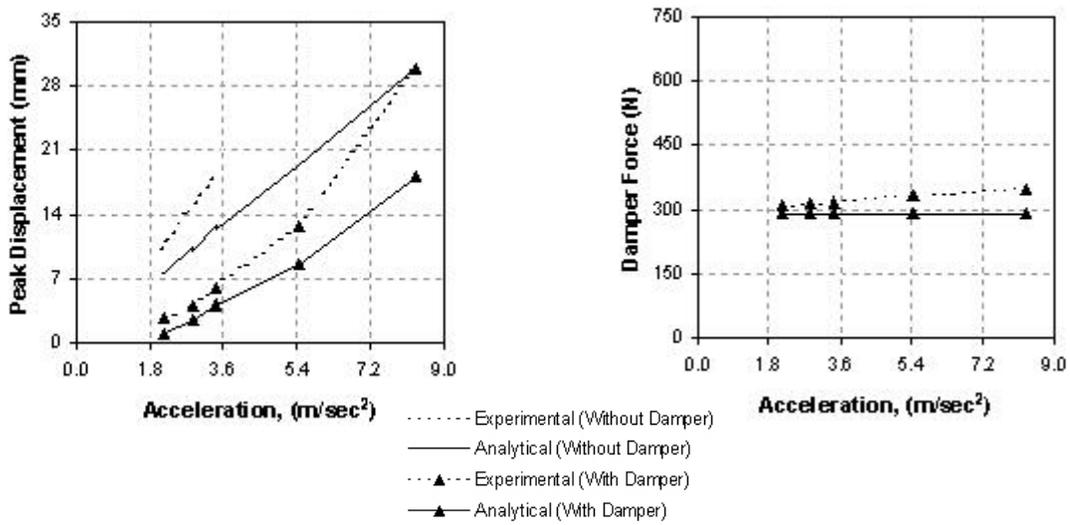
Figure 7. Seismic response in Z-direction of piping system with friction damper
