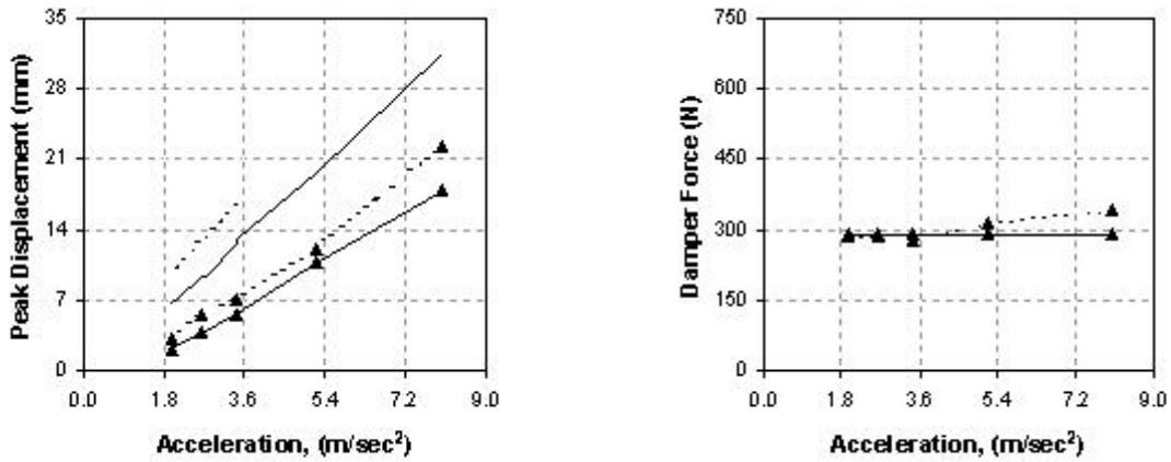
Figure 6. Seismic response in X-direction of piping system with friction damper
