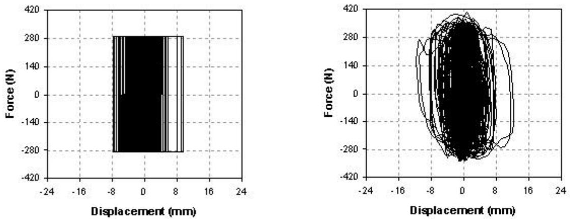
Figure 11. Hystereses for peak table acceleration of 0.53g in X-direction of the piping system
