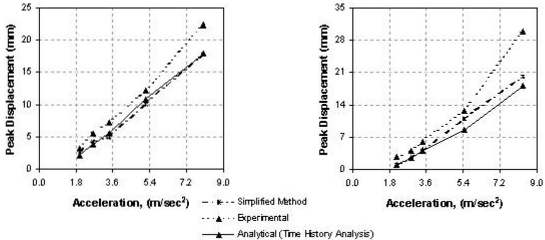
Figure 19. Seismic responses in X and Z-direction of the piping computed by simplified method
