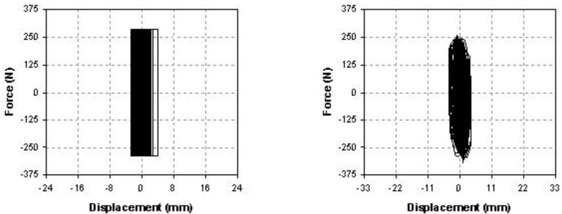
Figure 14. Hystereses for peak table acceleration 0.29g in Z-direction of the piping system
