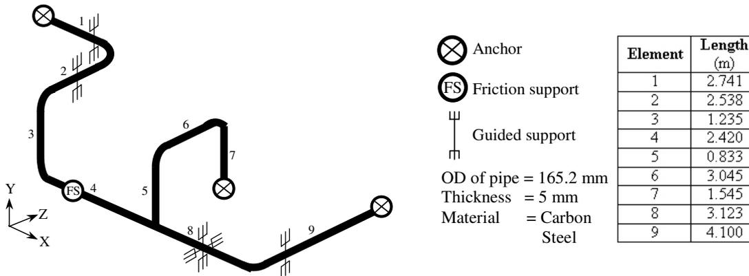
Figure 4. Schematic diagram of the piping system with friction damper
