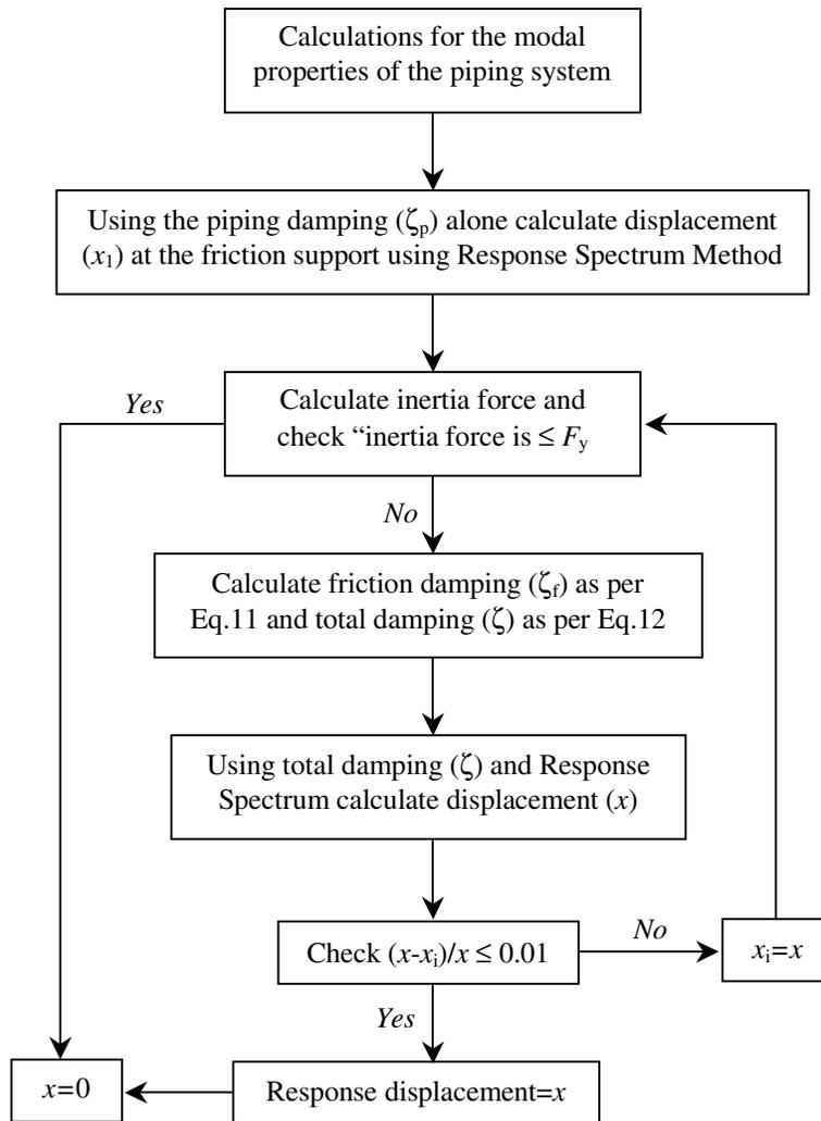
**Figure 18. Flow chart of the Iterative Response Spectrum method**
