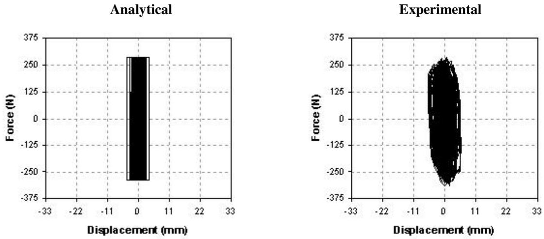
Figure 15. Hystereses for peak table acceleration of 0.35g in Z-direction of the piping system
