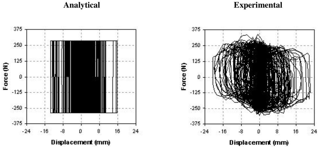
Figure 12. Hystereses for peak table acceleration of 0.82g in X-direction of the piping system
