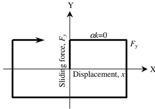
**Figure 5. Hysteresis for friction damper represented by Wen's model**
