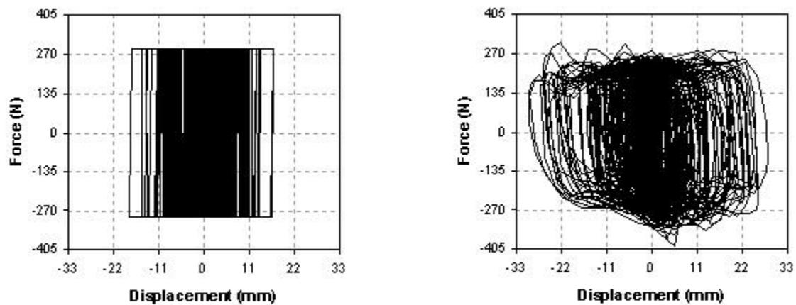
Figure 17. Hystereses for peak table acceleration of 0.85g in Z-direction of the piping system
