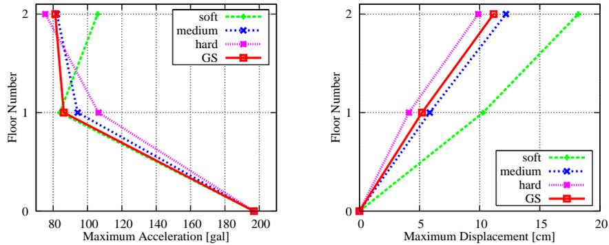
**Figure 13. Maximum Amplitude of Each Floor against Hachinohe Earthquake**
