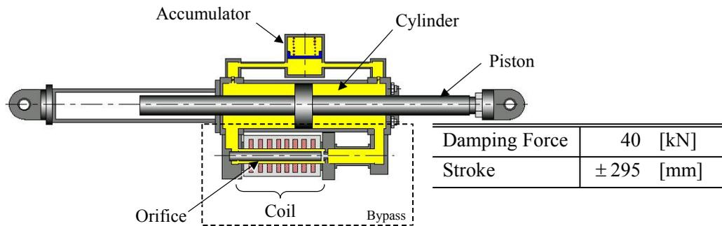
**Figure 3. MR Damper (MRD 40kN-590)**
