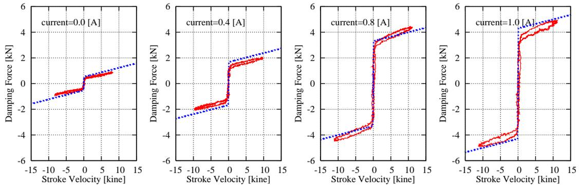
Figure 4. Characteristics of MR Damper
