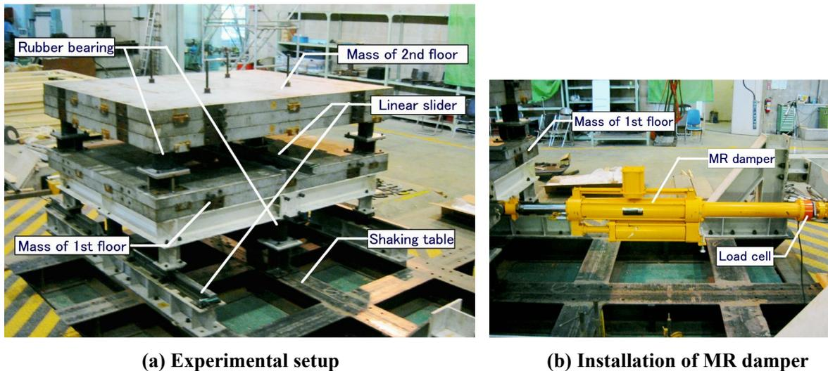
Figure 1. Experimental Setup and Numerical Model of Specimen
