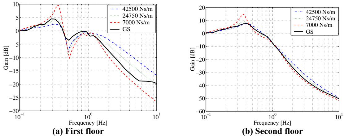
Figure 10. Frequency Responses of Mass Acceleration to Ground Acceleration
