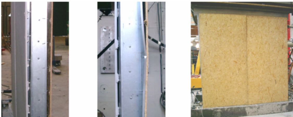
(a) Unzipping of sheathings (b) Distortional buckling of end studs (c) Wall deformation Figure 9. Specimen condition at failure in the case of the cyclic test.
