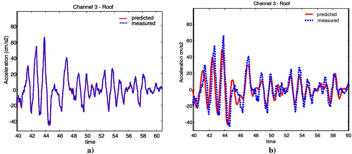
**Fig.3 a) Prediction using base motion and other output measurements, b) Prediction using base motion only**
