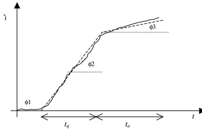
**Fig.4 – Schematic Illustration for the Running Integral of the Residual**
