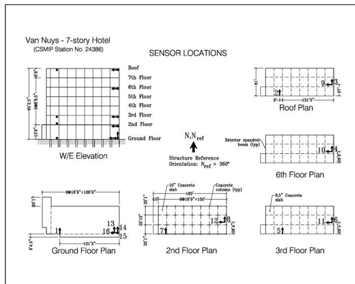
**Fig.6 Sensor layout (from CSMIP web site)**
