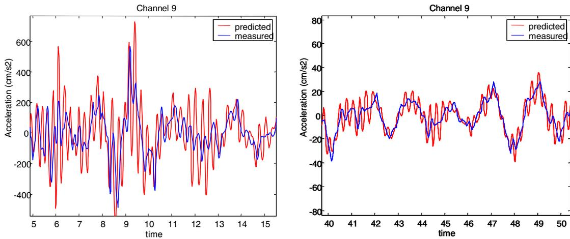
**Fig. 8. Comparison between the Predicted and the Measured Response for the building in fig.6 subjected to the Northridge earthquake**
