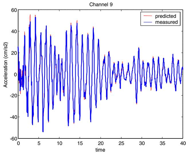
**Fig. 7. Comparison between the Predicted and the Measured Response for the building in fig.6 subjected to the Big Bear earthquake**
